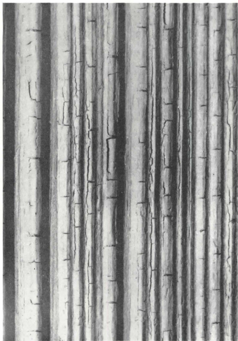
Stain (left) and shake paint (right) compared 18 months after start of weathering test made by Forest Products Laboratory. Latter shows considerable cracking and flaking. Stains use a lighter bodied oil—the best quality stains using a raw linseed oil.
