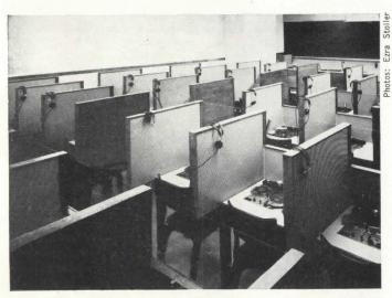
The language laboratory has 29 student positions in individual cubicles which house electronic equipment for listening and recording.
