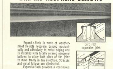
Expand-o-flash provides a continuous watertight seal all around the building both above and below grade.
