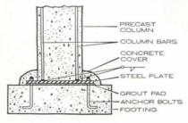
8 Precast column with a steel-plate base. Leveling nuts may be placed under the plate for convenience in erecting.
