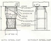
WITH STEEL CAP ULTIMATE LOAD: ULTIMATE LOAD: 262,000 LBS 50,000 LBS
