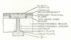
18 Precast girder, beam, and channel slab composite with in situ concrete. Bottom flange of inverted T-girder serves as seat for beams. Embedded steel in girder and beam joined by welding. Precast slab over the girder may be omitted, allowing a substantial in situ section to be cast as a composite top flange for girder and to provide space for placing negative reinforcing bars over beams and girders.
