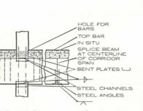
16 Precast beam connected to interior precast column. This detail is applicable to multistory construction where beams are continuous over the columns. Embedded steel in columns and beams is joined by welding. Negative reinforcing bars may be run through sleeve in column and covered with in situ concrete.
