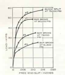
2 Pull-out test results. Bar sizes No. 5, 6, and 7 fully developed tensile strength and broke outside the concrete block. Block containing the No. 8 bar split vertically on all four sides when the steel tension reached 73,000 psi, and the bar, with grout and flexible metal tube intact, was pulled out of the block.
