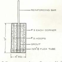
1 Pull-out test specimen. Concrete block cast with spiral flexible metal tube in center. Concrete  $f'_{o} = 6000$  psi. Tube was filled with neat cement-paste grout of thick consistency, and deformed reinforcing bar was placed by forcing it into the grout. Estimated compression strength of grout at time of test: 6000 psi.
