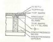
19 Section through beam and slabs of scheme shown in 18. Negative bars projected from ends of precast channel slabs are are welded together, and space over the beam is filled with in situ concrete.
