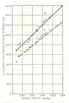
4 Ultimate concrete shear strength of composite specimens with varying percentages of reinforcing steel projecting across the joint face. Specimens are delineated in 3.
