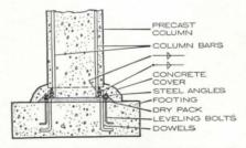
9 Precast column with an angle-bar collar at the base. Column bars are welded to angle, and, after erection, footing dowels are welded to opposite side of angle. This connection is advantageous where high-momentresisting joint is required.
