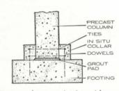
6 Precast column on footing with accurately placed grout pad. Grout pad is allowed to harden before setting column. Base of column is cast square and flat. In situ collar (cast-in-place concrete) is placed after erecting and bracing column.
