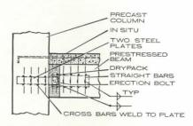
15 Precast beam connected to column by erection bolt prior to welding. This connection is advantageous for multistory construction as it speeds erection. Space around the welded connection is reinforced with suitable hoops and filled with drypack or cast concrete. Frame action may be developed by extending bar from column over beam and covering with in situ concrete.
