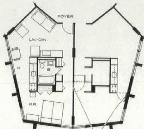
HINGED PANELS FOR CONVERTING TWO 1-BR. UNITS TO ONE 2-BR. UNIT AND ONE 0-BR. UNIT
