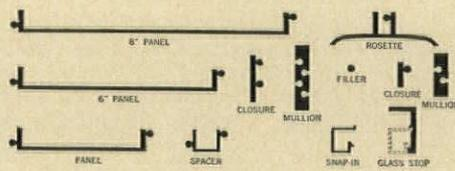
*Elements of Curtainscreen are 4", 6", 8" panels, mullions, spacers, and closures, fillers, snap-ins, glass-stops and rosettes. Other materials may be incorporated in framing system.*
