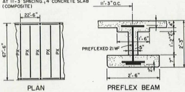
TYPICAL BAY: 67 FT STEEL BEAMS AT 7'-6" SPACING, 4" CONCRETE SLAB (COMPOSITE)
