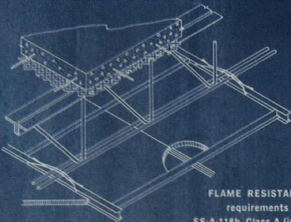
**FLAME RESISTANCE:** Meets requirements of Fed. Spec. SS-A-118b, Class A (incombustible). Two-hour fire-rated assembly.
