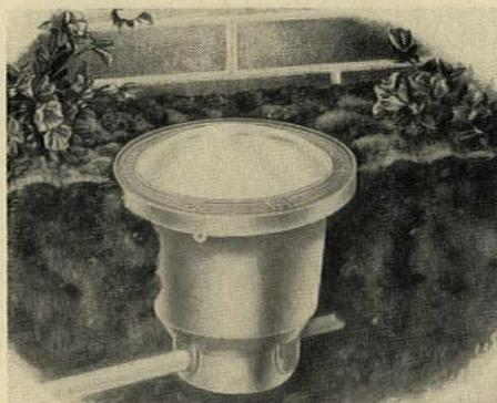
sion resistance, and the unit is fully sealed to meet all weather and grade conditions. Fixture is designed for 150 x PAR-38 flood or spot lamp, sealed beneath a clear-crystal tempered lens. Internal adjustment permits aiming of lamp in any direction up to 30 degrees off the vertical. Prescolite Manufacturing Corporation, 2229 Fourth St., Berkeley, Calif.
