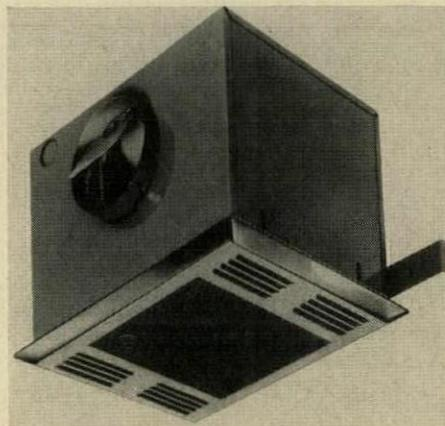
cycles. Heating elements produce both radiant and convection heat, and reach peak efficiency instantly. Housing is equipped with an adjustable bar for mounting between joists. Trade-Wind Division, Robbins & Myers, Inc., 7755 Paramount Pl., Pico Rivera, Calif.
