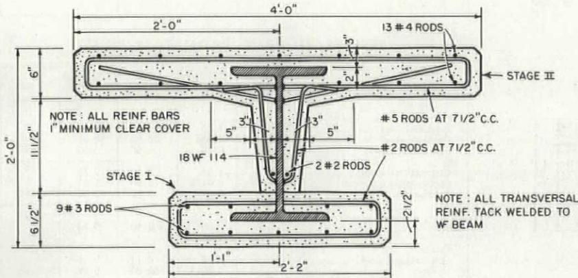
CROSS SECTION OF "PREFLEX" BEAM "PX-1"
