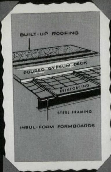
*Insul-Form*<sup>®</sup> offers great advantages as formboards in poured gypsum or lightweight concrete decks.
