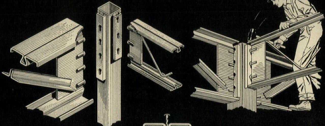
1. Completely interlocked members give unequalled framing rigidity and strength.
