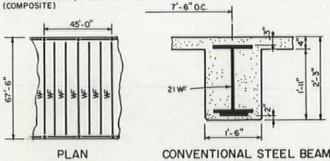
TYPICAL BAY: JOISTS AT 7'-6" SPACING PREFLEXED BEAMS AT 22'-6" SPACING 4" CONCRETE SLAB (COMPOSITE)
