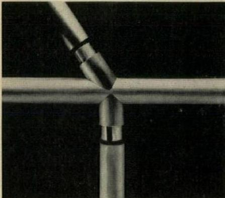
flush-type pipe railings without welds or exposed fasteners. Unlike conventional cast-aluminum fittings, the new connectors allow perfect color matches with pipe, even after aluminizing. Structural soundness and proper alignment are enhanced, since posts and top rails run in continuous lengths, uninterrupted by cross- and tee-fittings. Complete system, with all
