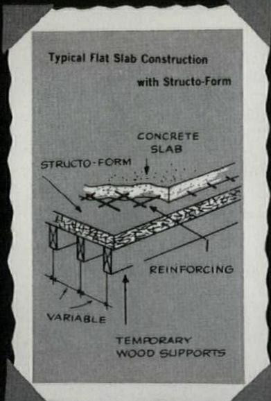
*Structo-Form*<sup>®</sup> provides uniform, lightweight, strong building planks for flat slab or reinforced concrete construction, producing a handsome finished ceiling.
