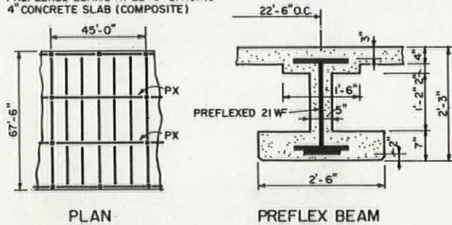
TYPICAL BAY: JOISTS AT 7'-6" SPACING BEAMS AT 22'-6" SPACING 4" CONCRETE SLAB (COMPOSITE)
