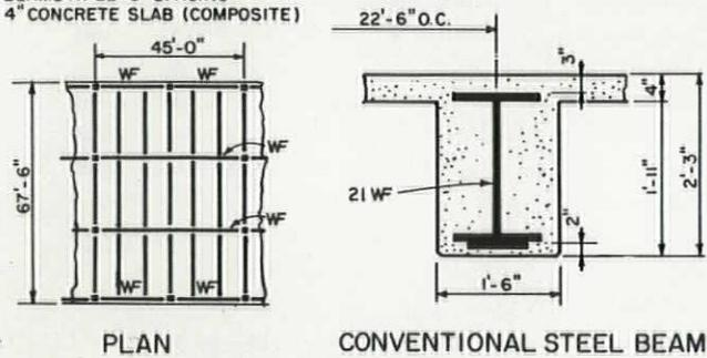
TYPICAL BAY: BEAMS AT 5'-7 1/2" SPACING, 2" CONCRETE SLAB (COMPOSITE) PREFLEXED GIRDERS AT 45'-0" SPACING
