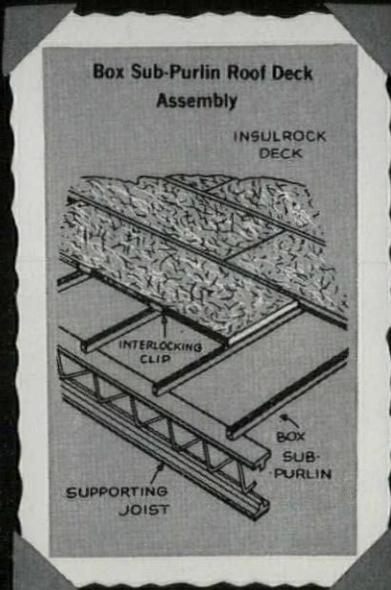
*Box Sub-Purlin* assembly gives new flexibility to open construction design, reduces costs.
