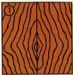
1. CENTER MATCH. Two consecutive pieces of veneer, one of which is turned over, are arranged side-by-side so the joint falls in the panel's center.
