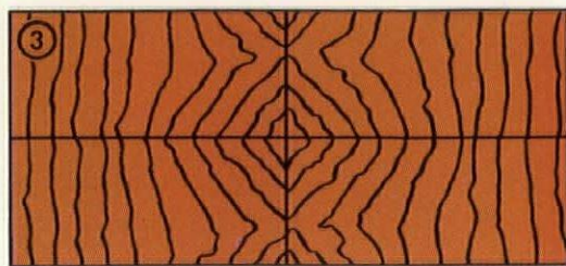
3. FOUR-WAY CENTER AND BUTT. This type of match is frequently applied to butt, crotch, or stump veneers, since it effectively reveals the beauty of their configurations.
