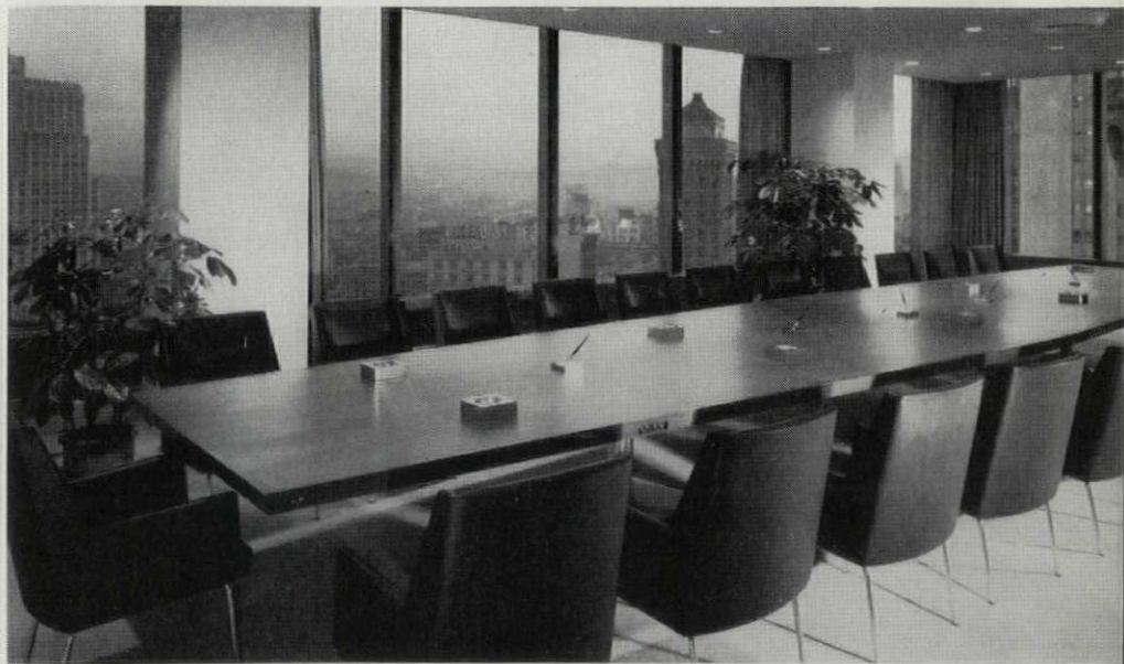
The board room is a bright and cheerful place to work because of the wide expanse of window area. SOLEX heat-absorbing glass used here absorbs about 50% of direct solar radiation and reduces glare.
