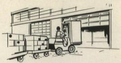
Faster Loading, Unloading. Small radio units give fork-lift truck drivers remote control to open and close doors they must pass through many times each day. Time saved in stopping, getting on and off truck and waiting for door to operate, can greatly reduce materials handling costs.
