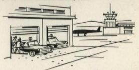
Airport Emergency. Combining electronically operated doors with emergency alarm signals saves valuable seconds for many airport fire stations. A signal from the airport tower simultaneously opens doors, turns on lights and triggers alarm bells in fire station often located at other end of airfield.
