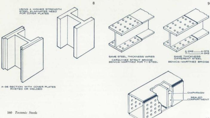
use of the material, and to simplify fabrication and maintenance, by welding diaphragms or bulkheads near the ends of the members, thus sealing the ends of the members and inhibiting internal corrosion. As a result, the only internal surfaces requiring maintenance painting are at the joints, thus reducing long-range costs as well as the initial cost. The bulkhead of this boxed section and the end connection for field bolting are shown (10).
