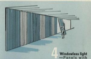
translucent plastic skins are completely interchangeable with aluminum or steel panels... enable the designer to turn whole wall areas into windowless, insulating natural light sources.
