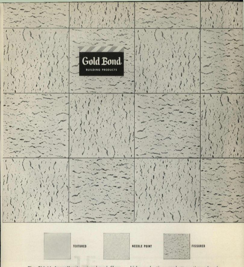
**Fire-Shield Acoustiroc's** mineral-wool fibers are *felted* for extra strength and stability. The long fibers are *interlocked*. Acoustiroc has 500% greater resistance to sag, 100% better dimensional stability, and 50% more strength than non-felted mineral wool. As a result, this 12" x 12" tile can be safely installed before plaster and terrazzo work are dry, to save seven days, or more, in building time.
