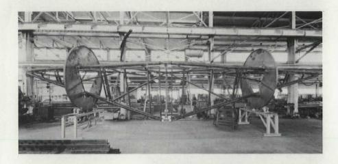
During fabrication process, large turning rings were attached to each end of tetrahedron enabling it to be rotated for down welding (above). Ladders inside tetrahedrons (right) were useful in skin erection and assist subsequent maintenance.
