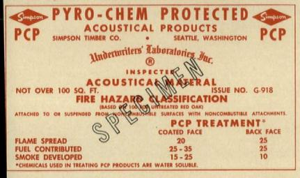
Now, on your very next job, you can specify Simpson woodfiber tile containing amazing PCP-and get Type 1 flame spread safety with up to  $\frac{1}{3}$  savings on material cost. PCP (Pyro-Chem Protection) — another revolutionary new product from the Simpson research laboratories—is a unique process that gives Simpson woodfiber tile a flame spread rating
