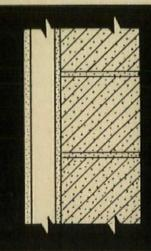
MASONRY WALL INSULATION Styrofoam insulation eliminates the need for furring and lathing. A new Dow method of quick installation permits adhering Styrofoam directly to the masonry, followed by the application of gypsum wallboard without the use of nails... or plaster can be applied directly to the face of the insulation.
