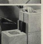
Strength with flexibility—the two basic factors for a repair-free masonry wall are assured by these engineered companion products. Dur-o-wal reinforcement, top left, increases flexural strength 71 to 261 per cent, depending on weight Dur-o-wal, number of courses, type of mortar. The ready-made Rapid Control Joint, beneath with its neoprene compound flange flexes with the wall, keeps itself sealed tight.
