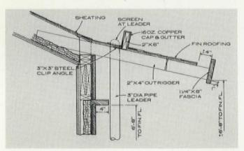
and gutters for widely overhanging roofs, for example, is both ingenious and handsome. A copper-capped 2" x 6" placed on end at the building line, and repeated use of the copper capping at the up-ended ridge beam, gives the roof a graceful, almost oriental, line.
