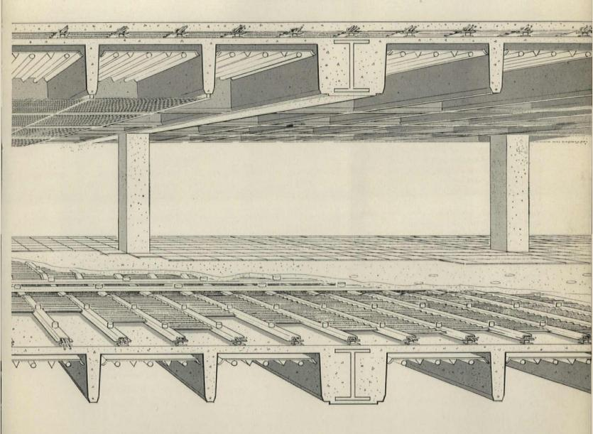
The plenum can be varied in height to meet any capacity requirement. Baffles zone air to desired areas. Adjustable supports assure level finish floor, compensating for dead load deflection and irregularities in structural slab.
