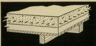
COMBINED FORM LINER/INSULATION. Styrofoam insulation eliminates the need for a form release agent . . . acts as its own vapor barrier . . . and provides high, permanent insulating values. Concrete keys positively to the cellular surface of Styrofoam insulation. When forms are removed, permanent insulation is in place, ready for finishing.
