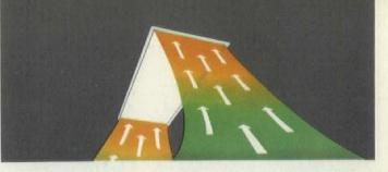
Reduce space cooling problems appreciably by extracting lighting heat before it enters the room.
