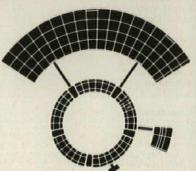
Office building, 238' ID and 344' OD, provides 137,000 square feet in five three-story sections separated by five four-story cores. Offices are in the sections: cores contain stairways, elevators, rest rooms, lounges. Fourth-floor penthouses are mechanical and electrical rooms. Sections are faced with precast panels and mullions of exposed quartz aggregate combined with white Portland cement. Cores are faced with
