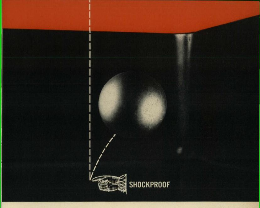
**DURCON® LABORATORY SINKS** can take it. As shown above, our quality control engineers drop a 3-lb. steel ball into Durcon sinks from heights of 6 to 9 feet. These tests prove Durcon resists impact blows far greater than those encountered in normal lab service.
