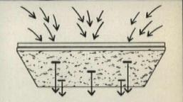
Heated or cooled air from the plenum passes through suspended Acoustone Tile, via openings designed to assure proper penetration of air and optimum comfort level.
