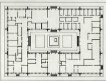
The plan of the Administration Building (above) illustrates the adaptability of the basic 60' x 68' space module. Offices are entered by way of the central court (top photo), paved in brick and concrete.
