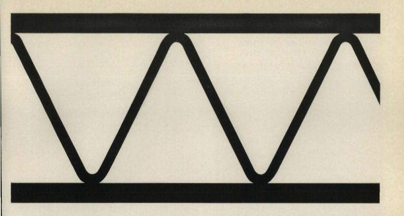
Available in lengths from 8 to 144 feet, in depths from 8 to 72 inches. Completely standardized and designed in accordance with SJI specifications.
