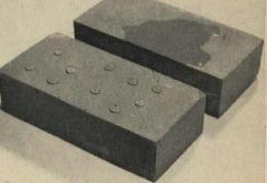
Note revealing contrast in water penetration of these two high suction rate brick. Water dropped on Silaneal-treated brick, at left, beads up without penetration. Same amount of water has spread rapidly across untreated brick, will be totally absorbed within seconds.
