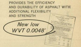
\*...grains/per square foot/per hour as measured in accordance with ASTM designation E96-53T, Procedure A. Tests conducted by the Chicago Paper Testing Company, Chicago, Illinois...copies available on request.
