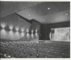
The sinuous pattern of the auditorium walls (above) is produced by the overlap of two surface treatments used for acoustical purposes—hardwood battens over glass fiber, and vertical boards. Steps along the entire front of the stage are convenient for many school functions.
