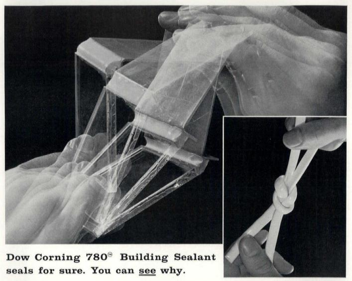
No other building sealant approaches *silicone rubber* for retention of *flexibility and adhesion*. That's the basic reason 780 Building Sealant *permanently seals* any combination of structural materials under temperature conditions ranging from —80 to 350 F. Note glass to aluminum bond above.
