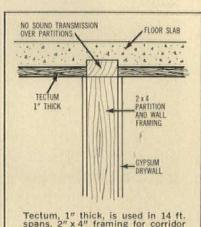
Tectum, 1" thick, is used in 14 ft. spans. 2" x 4" framing for corridor and party walls is cast into the concrete slab.
