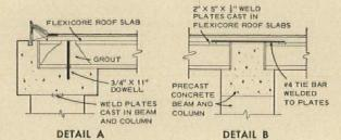
New Hi-Stress Flexicore slabs use high-tensile 7-wire stressrelieved strands to produce fully prestressed units. These slabs provide long, clear spans, high load carrying capacity and give improved performance.
