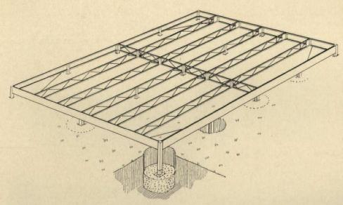
A new steel foundation system that will permit all-weather house construction has been announced by U.S. Steel. The foundation consists of 4 cold-formed "C-shaped" steel perimeter beams, 15 support posts, 4 diagonal corner braces, and 12 interior steel joists. In construction, perimeter beams and posts are assembled on the ground by mechanical fasteners, then tilted into position in holes 24" in diameter which have been augered to below frost line. Corners are then
