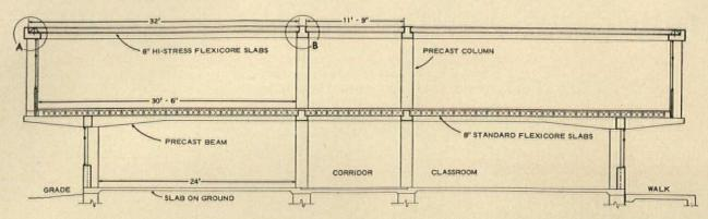
LATERAL SECTION. Hi-Stress Flexicore slabs, 32' in length, are used for long-span ceilings on second floor of class-room wing of Rutherford B. Hayes High School, Delaware, Ohio. The entire frame is precast concrete columns and beams.
