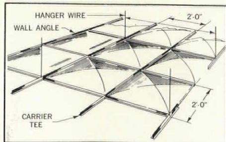
Installation of lay-in Textured Vault Panels is fast and simple in an exposed grid-type suspension system.
