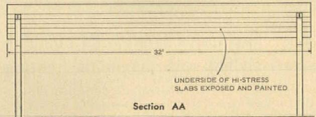
**ONE-STORY COMMERCIAL BUILDING ROOF DESIGN** requires only a steel frame on each side of the building to carry 8-inch Hi-Stress units on long clear span. Design can be repeated in any direction for larger building. Underside of slabs was exposed for neat, maintenance-free ceiling.
