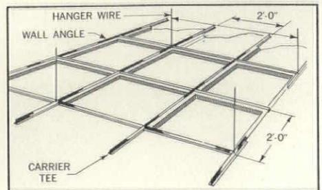
*Lay-in Inverted Coffier Panels are quickly installed in an exposed grid-type suspension system.*
