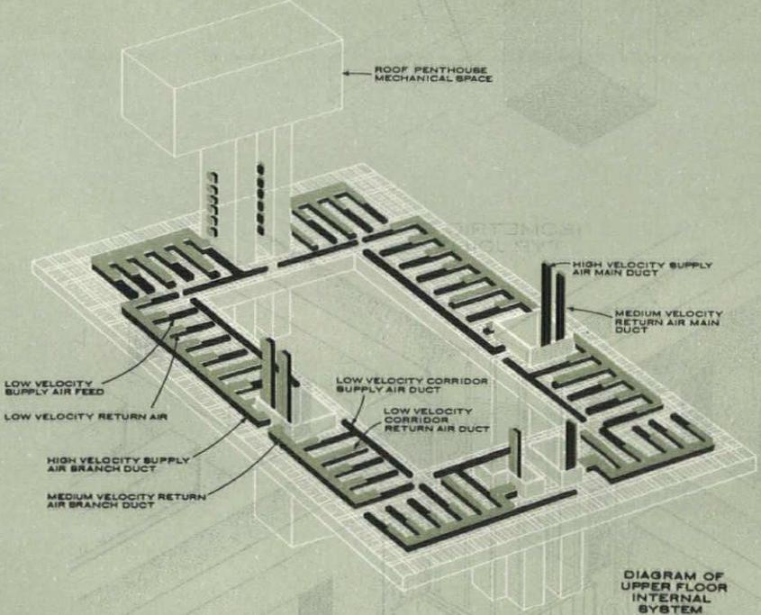
DIAGRAM OF UPPER FLOOR INTERNAL SYSTEM
