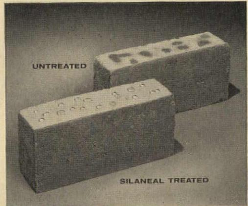
**Proven By Tests** Hundreds of transverse pressure tests — and tests simulating wind-driven rain — have demonstrated that wall sections built of Silaneal-treated high suction brick prove stronger and resist leakage better than similar untreated brick.
