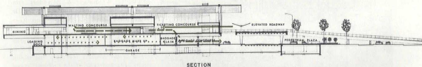
relatively economical, fireproof means of spanning the 30' x 120' bays; it permits the development of mezzanine spaces and has considerable visual impact. Roofing of white plastic and marble chips has been used to maintain the visual effect of the structure when seen from the air.
