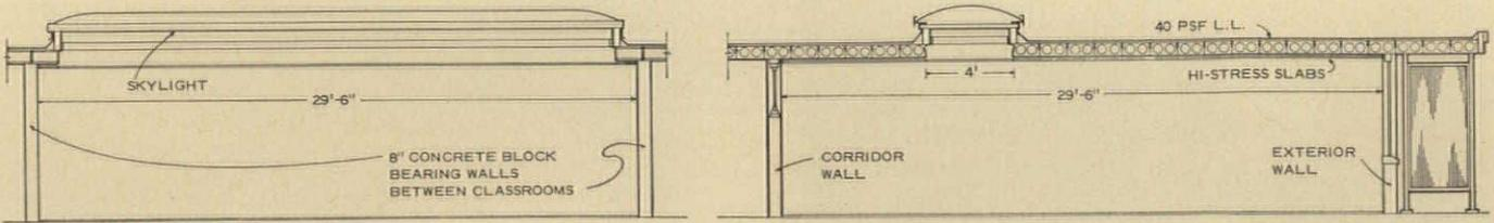
**SCHOOL WITH CLASSROOM SKYLIGHTS.** Flexicore Hi-Stress slabs with two  $\frac{7}{16}$ " stress-relieved strands clear span the 29'-6" width of the rooms, are designed to carry 40 psf roof load. Four slabs, two on each side of skylight, have three  $\frac{3}{8}$ " strands to carry the extra load of the skylight.
