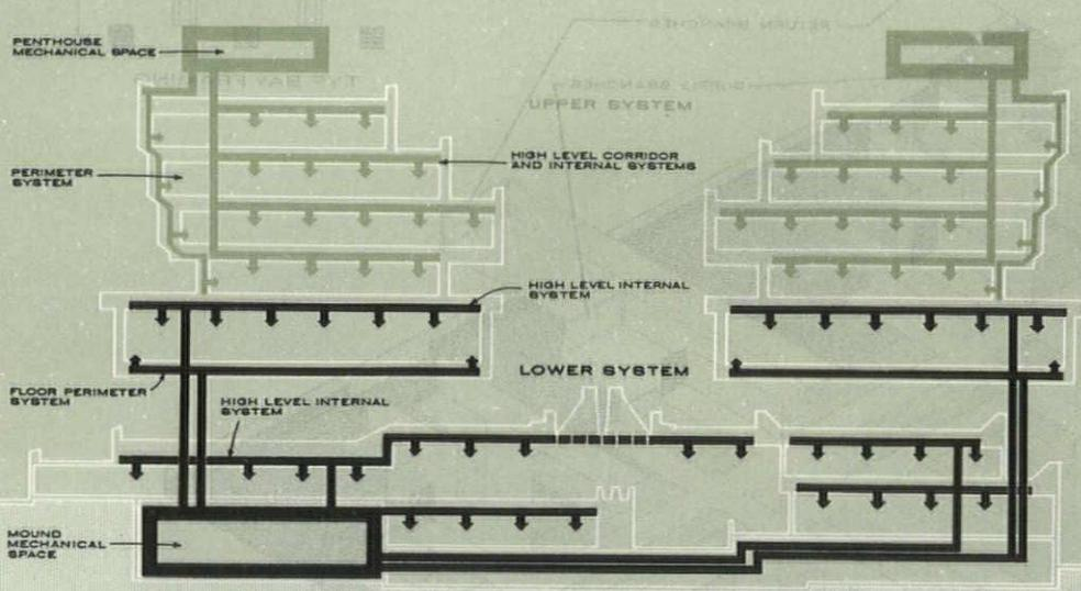
system, which is parallel to the supply, originates at low pressure and has a transition to high-velocity mains through attenuator and air valves.
