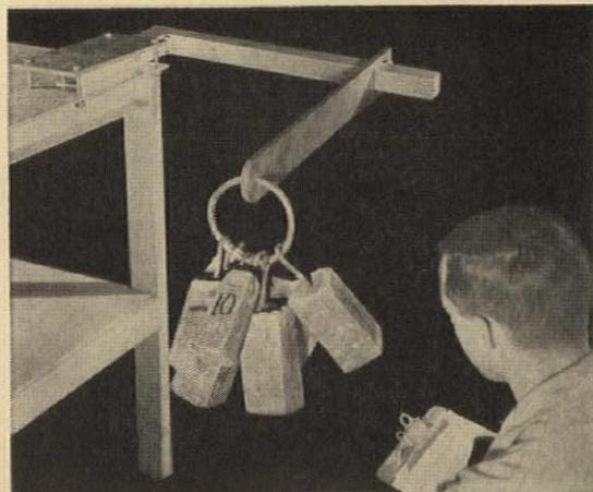
**Dual-Moment Lever Arm and Torque Test . . .** Simulates the most common, failure-causing loads submitted on door corners.
