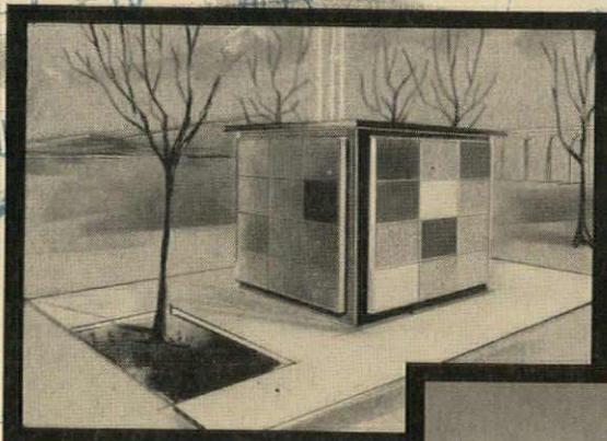
L-M's proposed design of a Transclosure® to house transformers and other electrical equipment. An example of the styling L-M can supply when the need arises.
