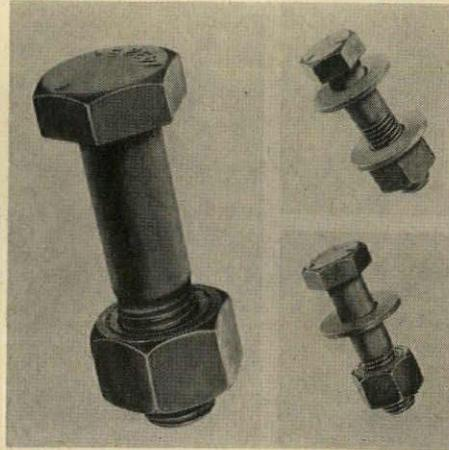
washers can be eliminated when tightening is by the turn-of-nut method, and when using heavy hex structural bolts in combination with heavy hex nuts. Two new economies result: cost of washers is eliminated, and shorter bolts can be used to connect the same thickness of material.
