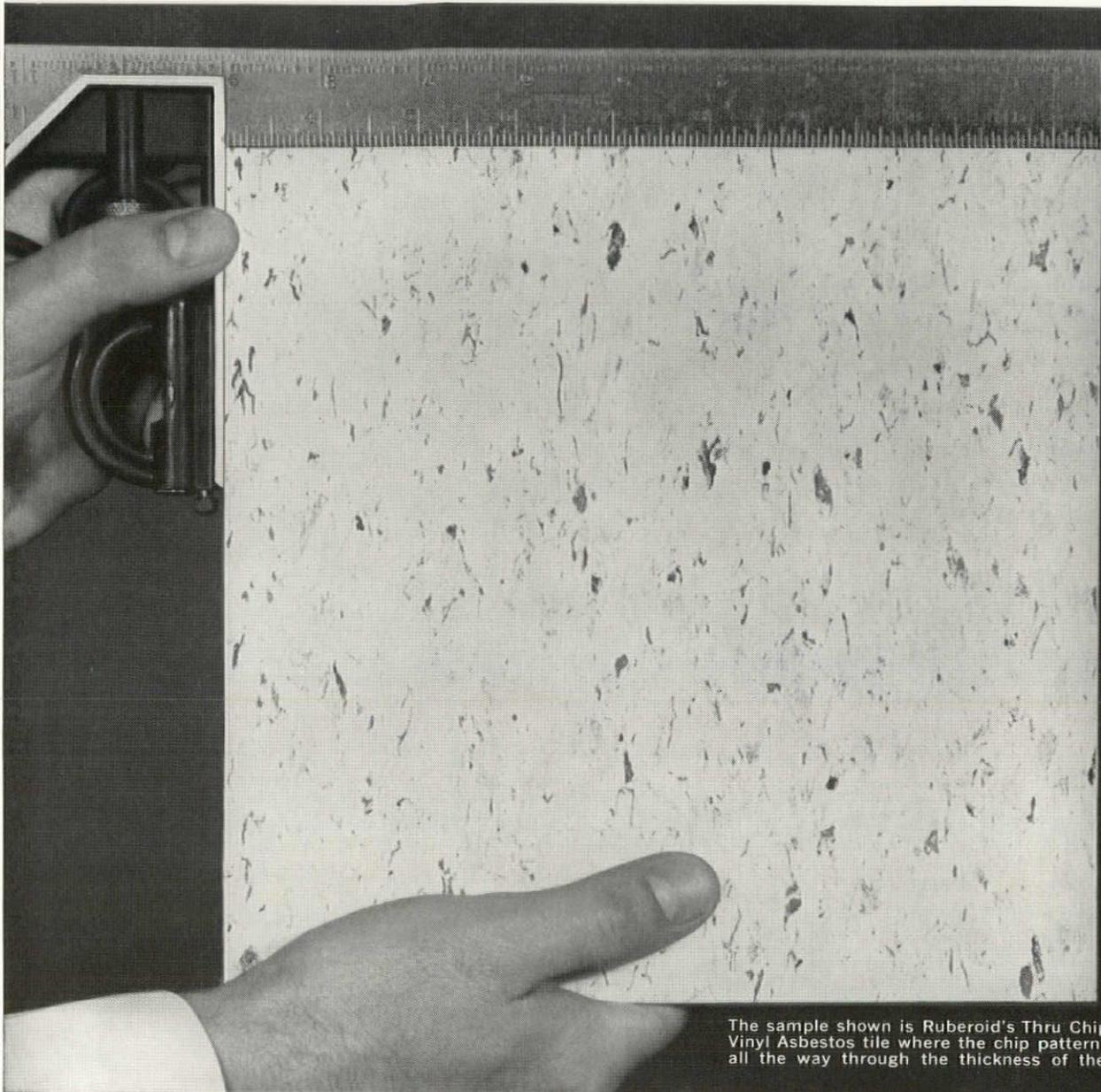
The sample shown is Ruberoid's Thru Chip, the Vinyl Asbestos tile where the chip pattern goes all the way through the thickness of the tile.
