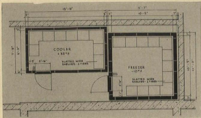
Plan view of two Walk-Ins, one a normal temperature and the other a low temperature, installed at Dobyns-Bennett High School, Kingsport, Tennessee.
