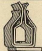
Heavy-duty phosphor bronze contacts are reinforced with spring steel clips that will take an 8-pound pull without detent.
