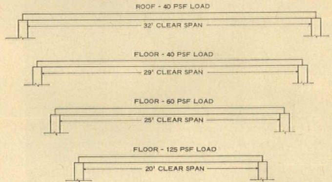
**TYPICAL LOAD AND SPAN** combinations for 8 x 16 Hi-Stress Flexicore slabs. Superimposed loads shown may be increased with composite design.
