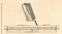
in three sizes to accommodate 2 x 6, 2 x 8, 2 x 10, and 2 x 12 members. Manufacturer states that the connectors will save up to \$30 or more per house by utilizing more effectively wood floor joist materials. Timber Engineering Co., 1619 Massachusetts Ave., N.W., Washington 6, D.C.
