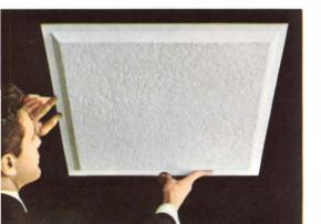
cost. Square lay-in panels are moulded in inverted coffer shape, projecting 2" downward into the room. As shown above, the visible surface has an attractive, low-relief, rippled texture. Panels are factory-painted white, but can, of course, be repainted to suit any decorative scheme. Measuring 24" x 24" x 2" deep and acoustically effective (NRC of .75) . . . Inverted Coffer Panels suggest interesting applications in supermarkets and other broad-expanse areas.
