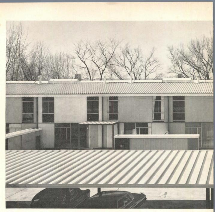
All structures in this new garden apartment complex are roofed with Armco ALUMINIZED STEEL Type 2.
