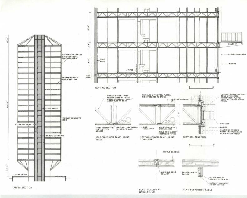
ing, but would offer the possibility of adjusting the prestress to take unequal loads on either side of the core, and carry unsymmetrical buildings with equal stresses. The top section of the core would be reinforced to take the cable pull; the bottom section would be widened with precast fins to provide greater lateral force resistance at the base.
