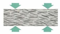
The fibers are air felted and mat formed by Weyerhaeuser's Patented Dry Process into a continuous blanket which is compressed under heat and pressure into panels. Natural wood lignin is the basic binder.
