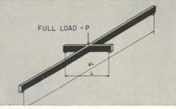
The action of a one-way floor is typified by this framework which has a high ratio of long to short span.
