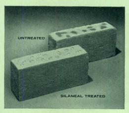
Proven By Tests Hundreds of transverse pressure tests — and tests simulating wind-driven rain — have demonstrated that wall sections built of Silaneal-treated high suction brick prove stronger and resist leakage better than similar untreated brick.
