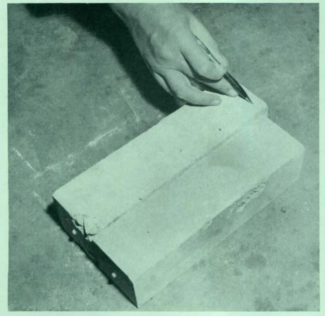
Expansive concrete's growth is illustrated by these two test samples. One was cast with ordinary concrete, and the other (longer) with concrete containing about 15 per cent "expansive component" in the cement.
