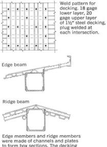
were made of channels and plates to form box sections. The decking was connected at the beams by welding to pipe sections and angles which formed easy-to-weld seats.
