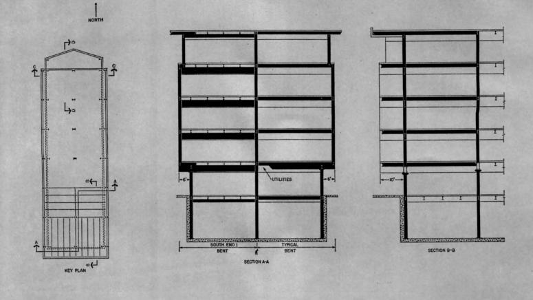
In the unique design of the Allentown City Hall and Police Building, the main tower is cantilevered at the second floor on three sides—6 feet on the east and west, and 10 feet on the south.
