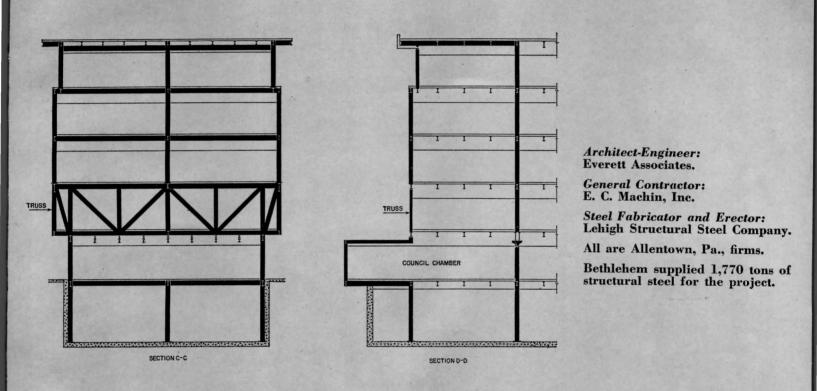
10-ft cantilevers on south . . . solved by steel The 10-ft cantilever on the south side, and the two-way cantilevers required at the corners (see key plan) were solved by dropping the girders in the southernmost frame, thereby allowing the filler beams to pass over the girders and develop the cantilevers rather simply at each floor. (See Section B-B.)
