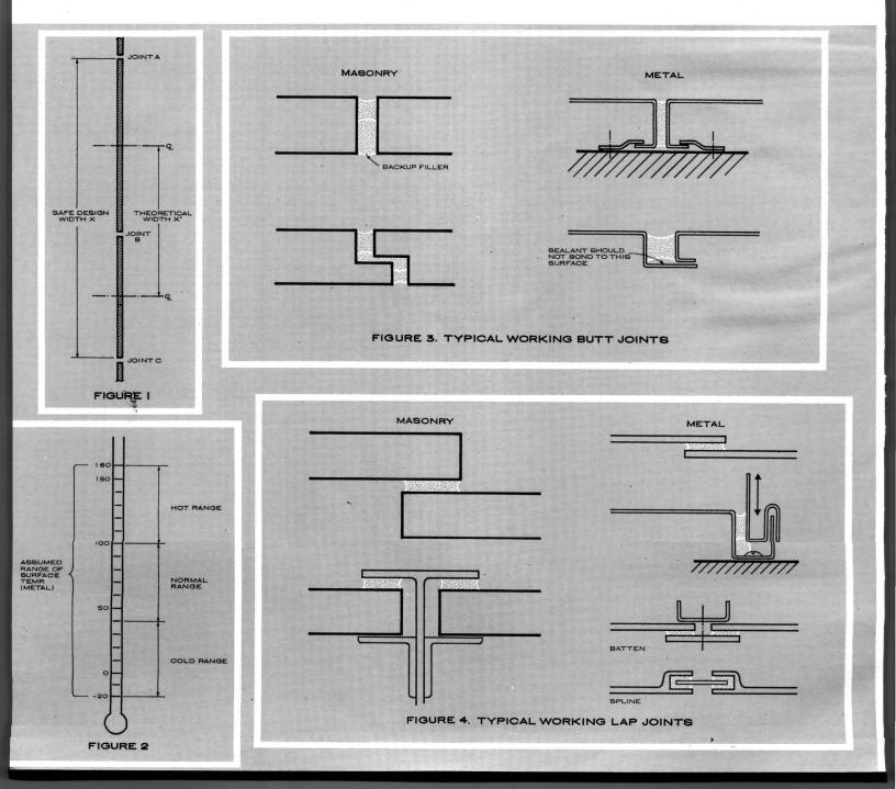
metals is indicated diagramatically (2), divided into three sections designated as the cold, normal, and hot ranges. Note that the temperatures indicated do not refer to the ambient temperature, but to the surface temperature of the material.
