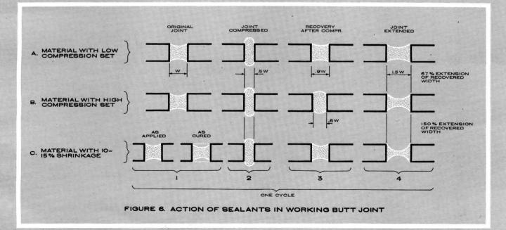
material A is extended by only about 67 per cent of its recovered width to reach the same joint dimension. The disadvantages of materials that shrink noticeably upon curing are illustrated in line C. It will be seen that when such a material is extended by the required 50 per cent of the original joint width, high tensile stresses are imposed on the small neck section, inviting rupture.
