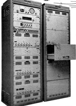
**CENTRAL CONTROL UNIT** contains power source for entire sound system. It also has three self-contained program sources – AM/FM tuner, record changer and a Webster Ekotape® recorder-reproducer.
