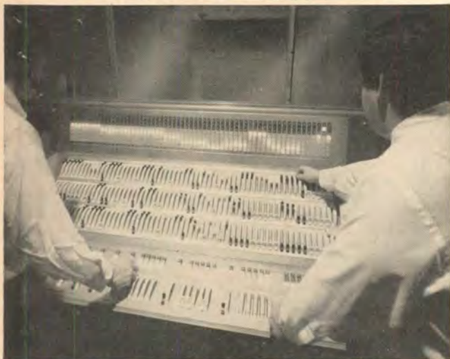
Even the most complex light plot has not required more than one student operator for this SCR® dimmer control
