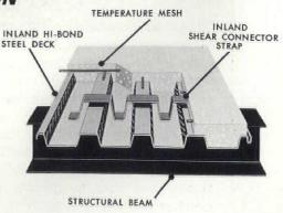
ALTERNATE: INLAND SHEAR CONNECTOR STRAP is welded through Inland Hi-Bond Deck to the beam below.
