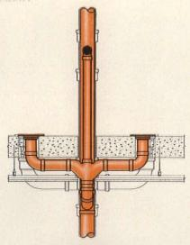
SAVES BETWEEN-FLOOR SPACE. In this layout, the use of compact, space-saving copper for the sanitary drainage system saves 5½" of building height per floor. In a multistory structure, this could mean thousands of dollars saved in construction materials and labor.
