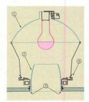
SILVER BOWL REFLECTOR (1) Total light is directed upward to ellipsoidal Alzak® reflector which focuses light through(2) small molded black phenolic cone aperture—retained in (3) reversible (Duo-Cast) die cast trim. (4) Spring loaded latches permit removal of housing for access to splices and/or top relamping.
