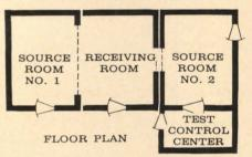
This floorplan illustrates how the laboratory is actually three individual buildings separated by insulating air spaces to eliminate sound transference from chamber to chamber. The major purpose of this modern up to date facility is to, by development-testing, improve the sound retarding qualities of the individual panels used in the construction of Folding Walls... and
