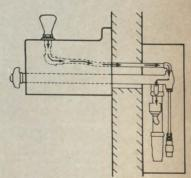
No cutting or fitting of frostproof valve assembly required on job site. Fountain and valve ready for ipstallation. A 1¼ ° O.D. drain tube elbow is provided with extra length to allow for exact cutoff (1-inch) entrance into interior plumbing cabinet. Valve extensions are made to customer's exact wall thickness.
