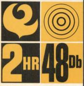
THE BASIC SYSTEM OF TWO LAYERS OF 1/2" TYPE "X" WALLBOARD ON STEEL STUDS GIVES YOU 2-HOUR FIRE AND 48-DECIBEL SOUND RATINGS!
