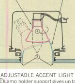
ADJUSTABLE ACCENT LIGHT (1)Lamp holder support gives up to 35° of vertical angle adjustment.(2) Molded, high heat aperture shield in (3) reversible (Duo-Cast) die cast trim (4) rotates through 358° horizontal arc with positive stop. Lamp/shield relationship consistently maintained. May also be used in sloping ceilings.
