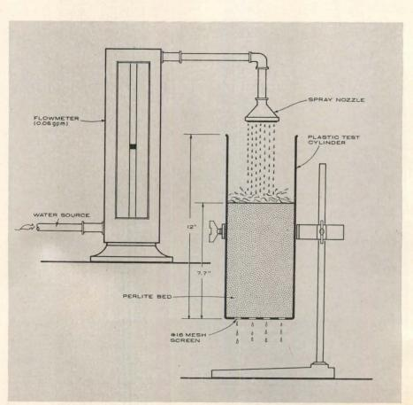
2. Johns-Manville Research and Engineering Center exposed silicone-treated perlite to 75 soaking and drying cycles in a flow-through test apparatus and concluded that it will maintain its water-repellency indefinitely.
