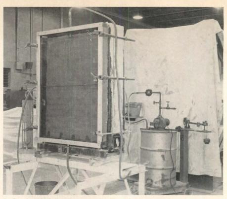
1. Tests by SCPRF show silicone-treated perlite insulation prevents moisture passage through a cavity wall and maintains constant insulating efficiency under wind-driven rain exposure.
