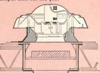
An optional in-the-roof sound attenuator—recessed to maintain unit's low profile—offers maximum quietness for sensitive areas of the building. This arrange-
