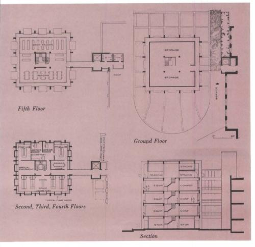
laboratory stories was required to make the floor levels correspond to those of the existing building. The seemingly superfluous building volume involved cost very little and is of value in minimizing air pollution in the labs.
