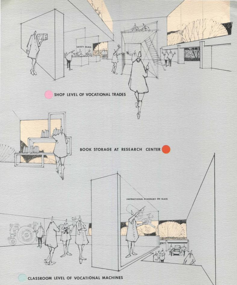
The TRADE AND INDUSTRY area is planned with a workshop well and related classrooms on the balcony. One-half-inch laminated safety glass partitions would separate machinery alcoves to isolate the noise and for visual student surveillance.
