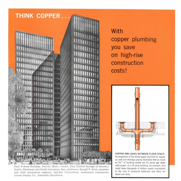
Described as Detroit's most distinguished building, the new twin tower First Federal Building is truly copper-protected—actually more than 4 miles of copper tube were used; Type L for hot and cold water lines in sizes  $\frac{1}{2}$ " to 3" and Type DWV for sanitary drainage in sizes up to 6". By specifying copper tube, the architects and mechanical engineers saved piping space, and cut installation time and costs throughout the 23-story structure.
