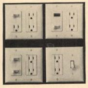
Line of "Medalist" combination devices have AC quiet switches and split circuit wiring. Devices contain break-off feature that permits 16 different wiring applications with only seven catalog numbers. Separate or common feed is available in one device. Other features include 20-carat goldplated switch contacts, com-pact body 1/4" shallower than other devices, and staked and backed out screws. Slater Electric Inc., 45 Sea Cliff Ave., Glen Cove, N. Y. On Readers' Service Card, Circle 115
