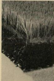
fibers electrostatically to jute backing - 17,500 individually applied per sq. in. The result is not a conventional flocked fabric nor a tufted or woven fabric; it is a velvet-type carpet, called "Veltron," of singularly lustrous texture (hence the 'Vel'; 'tron' is for the elec-tronic process). The <sup>1</sup>/<sub>5</sub>"-thick durable pile remains perfectly vertical and resists abrasion due to its unusual density. Color pattern is achieved by Colorset-Barwick's silk-screen
