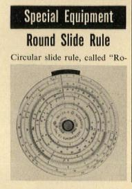
torule," permits one-hand operation and continuous readings. Slide rule has Pythagorean and Ei scales and is available in 3", 4", and 5" diameters with scale lengths up to 15.7". Manufacturer states that Rotorule costs less than 50 per cent of comparable slide rules. Scientific Instruments Co., 2126 6 St., P. O. Box 224, Berkeley, Calif.
