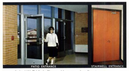
Series 1600 Tri-Style Closers with narrow, clean lines to compliment modern doors. Available in invisible mounting, back mounting and exposed mounting. PATIO ENTRANCE invisible top-jamb mounting with screws concealed. Closer body does not project past narrow top frame. STAIRWELL ENTRANCE exposed mounting with parallel arm for an attractive installation for even out-of-the-way places.
