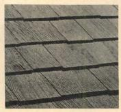
Mineral-based roof shingles are textured and colored to look like weathered cedar. They can be cut with a saw and nailed, but will not burn. Manufactured in 16" lengths, and in 6", 8", and 10" widths. Johns-Manville, 22 E. 40th St., New York, N.Y. 10016.
