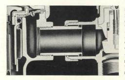
Sloan's New Adjustable Tailpiece slides in or out of the Control Stop until the desired roughing-in dimension is obtained. Tightening the coupling nut compresses the stainless steel split ring against the tailpiece until a rigid connection is made. The "O" ring provides a water-tight seal. There is no danger of over-adjusting. When the maximum adjustment is reached, the shoulder containing the "O" ring engages the stainless steel split ring and comes to a solid mechanical stop.
