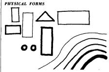
Building heights indicated by weight of the line: the heavier the line, the taller the structure. Topography similarly illustrated.
