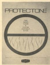
Fire ratings are given for "Celotex Protectone" ceilings using acoustical tile and lay-in panels. Data sheets chart ratings for various Protectone materials used in ceilings suspended from steel or wood joists supporting concrete or wood floors. Detail drawings. 39 pages. The Celotex Corp.,
