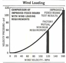
Results shown above are obtained under controlled laboratory conditions without consideration for the possible effect of air foil or other wind forces.
