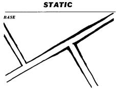
Paths: indicated by a double line that varies according to road width. Through line weight, the less dominant topographic characteristics are reflected.
