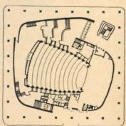
2400, 2000, and 1800. Ceiling panels can be lowered electronically to the balcony-rail level for the first seating change (3001 to 2400). For 2000, the mezzanine area will also be sealed in with panels. The minimum number of seats can be obtained by cutting off the last five rows of the orchestra floor.
