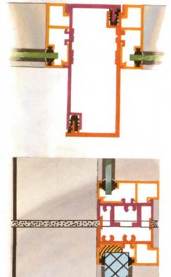
800 System Curtain Wall expands due to extreme summer heat . . . . . contracts due to severe winter cold . . . all expansion and contraction takes place within the module, both horizontally and vertically.
