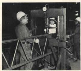
with high ampere-low voltage current and great pressure, forging the members into permanent union. Precise automatic control of current and pressure eliminate variation.
