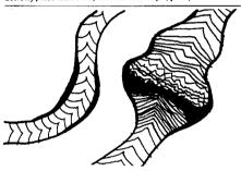
Water (in motion): direction of flow indicated by bend-ing the line used in "water contained." Speed (e.g., waterfalls and rapids) indicated by number of lines.
