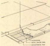
"Acoustipads" between gypsum board backing and standard acoustical metal pan assembly to reduce sound transmission. Perforated pan units are 1' wide by 1', 2', 3', or 4' long. Noise Reduction Coefficient range is .75 to .85. National Gypsum Co., 325 Delaware Ave., Buffalo, N.Y. On Readers' Service Card, Circle 100
