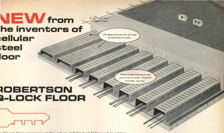
w Q-Lock Floor possesses all the virtues of Robertson Q-Floor while adding me new ones of its own. When concrete is poured over Q-Lock Floor, the entifically-designed indentations and embossments rolled into the steel actural elements develop composite action. Therefore, this new design locks ether the structural properties of both materials in a tight grip and results a more efficient and economical use of both materials. Use the coupon or te to Robertson on your letterhead for literature.
