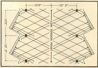
The tendons are placed diagonally on a one to two slope to the transverse column direction with the column strip tendons extending to the tips of the saw teeth. Structural analysis was based upon load balancing applied to a flat plate.
