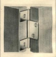
Three-leaf door hinge needs no mortising and shows knuckles on one side, and only leaf edges on the other. Brassplated steel hinge, "4741," measures 3<sup>11/32</sup>" long by 2<sup>9/32</sup>" wide open. Samples available. Amerock Corp., 4000 Auburn St., Rockford, Ill. 61101. Circle 109, Readers' Service Card
