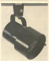
O-Flood is a wide-beam floodlight, using a 250-w miniature quartz iodine lamp. It is finished in jet black, bronze (both with black yoke and mounting), and matte white. A deeply recessed reflector reduces glare and spill light. Flow-through convection venting cools the lamp. Available with a variety of mounting devices (among them cclamp for pipes, screw-in unit for lamp socket), accessory louver, hood, and color filters. Lighting Services, Inc., 77 Park Ave., New York, N.Y. 10016.
