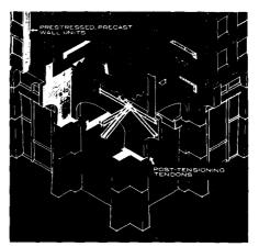
Combined stressing techniques enable contractor to stack prestressed, precast. . . .
