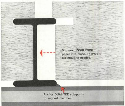
DUAL-TEE is the revolutionary new steel sub-purlin Flintkote designed to supplement the INSULROCK structural portland-cement-bonded wood-fiber deck system. The INSULROCK panels lock around the DUAL-TEE sub-purlins and butt together at the top. What's more, with all the time and money you save by not having to grout, you actually get better thermal insulation with the unbroken upper surface that only INSULROCK panels with DUAL-TEE sub-purlins provide.
