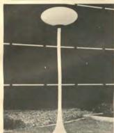
Plastic ellipsoid luminaire atop a cast-aluminum pole for outdoor lighting accommodates up to 400-w mercury vapor or 500-w incandescent light. Pole (8', 10', 12', or 14' high) is finished in baked acrylic — white, black, or dark bronze. Luminaire, 34" dia., has built-in reflector. Suitable for parks, campuses, parking lots, street lighting, etc. Kim Lighting, 1467 N. Lidcombe, El Monte, Calif. 91733.
