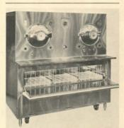
Cooker-freezer meets mass-feeding needs by cooking 40 lb of vegetables every 5 min or heating 48 frozen entrees every 6 min. Directly under the two steam cooking compartments ("400 steam jets impinging directly into the food mass for dynamic cooking action") is a 300-lb capacity freezer. The "2285-FC" virtually eliminates the need
