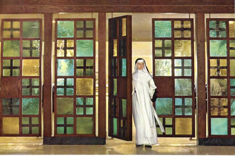
Main chapel entrance with stained art glass doors controlled by Norton Series 1940 overhead concealed double acting closers. These doors are very heavy and place an extremely high inertial load on the closers. In addition, a natural draft, due to the construction of the building, is always present. The doors are under control at all times.
