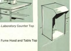
Nicolet's KolorMate, a monolithic asbestos-cement material, is fast becoming the first choice of architects, industrial designers, and laboratory planners for use in laboratory-furniture applications. KolorMate is well known as an acid and corrosion-resistant material which can be machined and cut using techniques common to stone fabrication.
