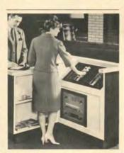
Control console for paging and radio sound distribution has AM/FM tuner and 10-station switch bank for zone paging. Compact unit is designed for central location such as front desks in motels or hotels. RCA Service Co., Dept. 1614, Bldg. 203-3, Camden, N.J. 08101.
