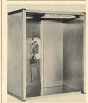
Compact phone "booth" is all stainless steel, including perforated acoustical side panels. Shelf unit accommodates the Bell System 235G Panel Telephone mounted either on the left (40-S) or on the right (41-S). Dimensions: 24" wide x 30½" high x 145/16" deep. Suitable for lobbies, department stores, etc. Manufacturer plans to offer a variety of side-panel finishes and various accessories. Acoustics Development Corp., 1810 Holste Rd., Northbrook, Ill. 60062. Circle 133, Readers' Service Card
