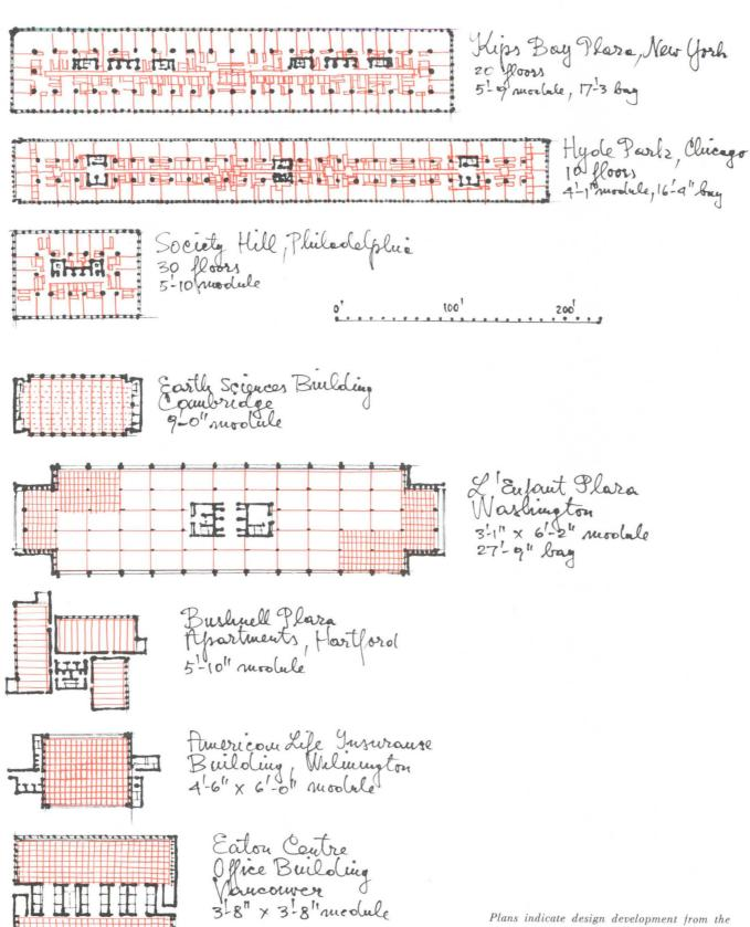
Christian Science Church Center Boston 4'-7/2" x 6'-2" module Plans indicate design development from the rigid approach based on conventional steel-framed structures to the simpler interiors of concrete loadbearing walls, and, later, fully integrated structures. The simpler layouts tend to produce a stronger architectural form.
