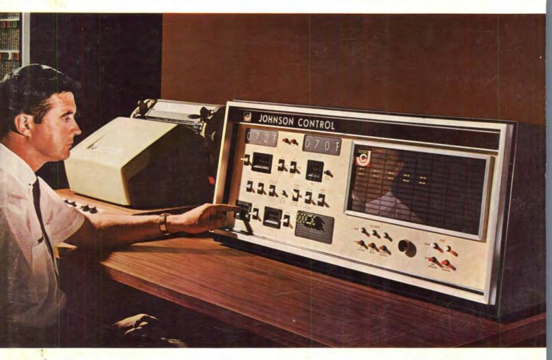
Our new solid state electronic control centers are the first to utilize economically all types of signals — pneumatic, electric and electronic. They cut the cost of remote reset and control and make it practical to centralize every function from air conditioning control to fire detection and illumination. One center can serve any number of buildings.
