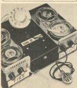
"Attention — an emergency message follows" . . . says the Dialalarm, which will automatically call emergency help should a piece of machinery fail, or a fire start. Wired into existing security systems, it will, for example, automatically call police and deliver its prerecorded message if a building is entered forcibly. The same unit will also call the fire department when acti-
