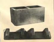
Building-blocks made from common soil with petroleum asphalt binders may eventually have far-reaching repercussions in the building industry. According to the developers, the Esso Research and Engineering Company, the blocks will cost from 2¢ to 5¢ less than comparable concrete blocks.
