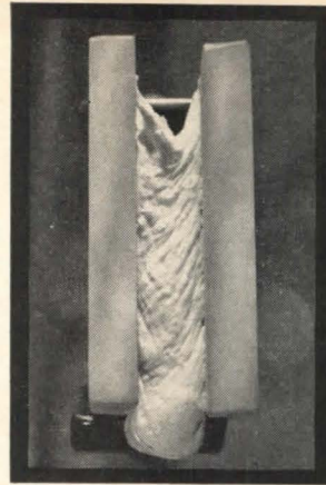
Acrylic sealant after 30 cycles in Joint Movement Simulator. Pumped out of place.
