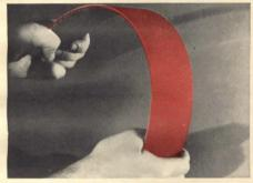
Permanently flexible. Made of silicone rubber, Traffic Topping keeps its resilience indefinitely. Won't harden, soften or become brittle, even at -65°F or 300°F. Provides a cushioned walking surface as
