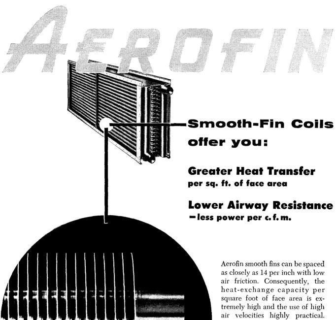
Tapered fin construction provides ample tube-contact surface so that the entire fin becomes effective transfer surface. Standardized encased units are arranged for simple, quick, economical installation.
