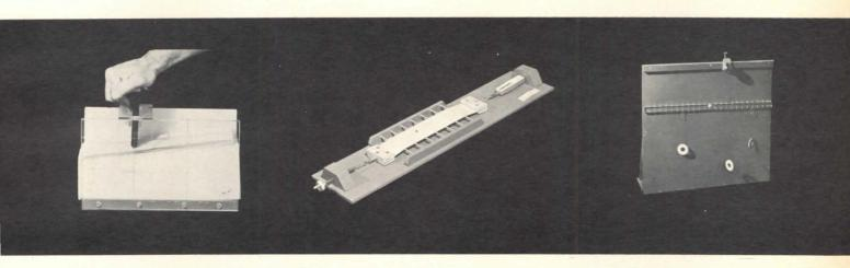
Center third: Applying a load within the center third of a rigid body compresses the base at all points. In model, load outside center third lifts foam rubber base.
