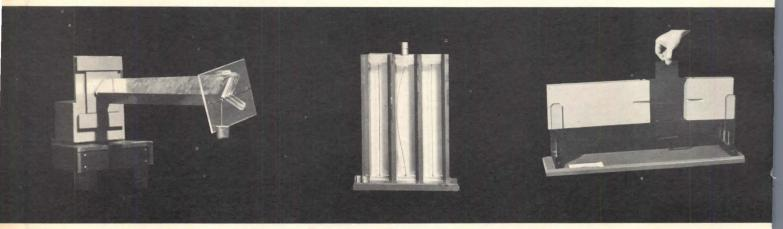
Shear center: Level bubble indicates when movable weight counterbalances twisting in a cantilevered member. The point of balance is the shear center of the member.
