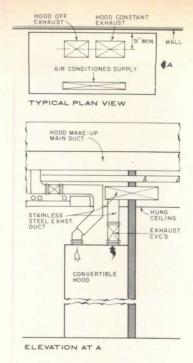
Air and exhaust ducts at typical fume hood.
