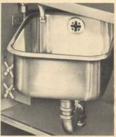
Swingaway sink. Stainlesssteel sink saves space by pivoting on its drainpipe under a counter. Bowl, 1634 x 11½" x 6" deep, is supplied assembled with overflow, drain, swivel joint, and bracket for wall mounting. Holderle Bros., 1214 Brooks Ave., Rochester, N.Y. 14619. Circle 124, Readers' Service Card
