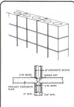
Concrete block is coming up in the world—and fast. These loadbearing walls of scored 8" x 8" x 16" block were completed at a rate of one story per week over a four month period, enabling the owner to open for the summer season. Note how transverse wall system provides the amenity of balcony privacy. Integral scoring treatment in the modular unit evinces a more attractive wall network of 8" squares. The loadbearing walls support concrete floor slabs that were precast at the site.
