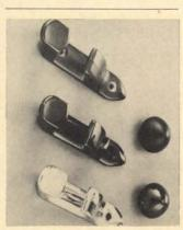
Black Chrome. DURAMIR BK, a black chrome plating compound, overcomes former difficulties of earlier experimental black chrome because it requires neither low temperatures (and consequent refrigeration equipment) or high current densities. To convert an existing system, a plater must simply add an extra tank with DURAMIR BK, which can be deposited over bright chrome or the final nickel plate. With the exceptions of aluminum and magnesium,
