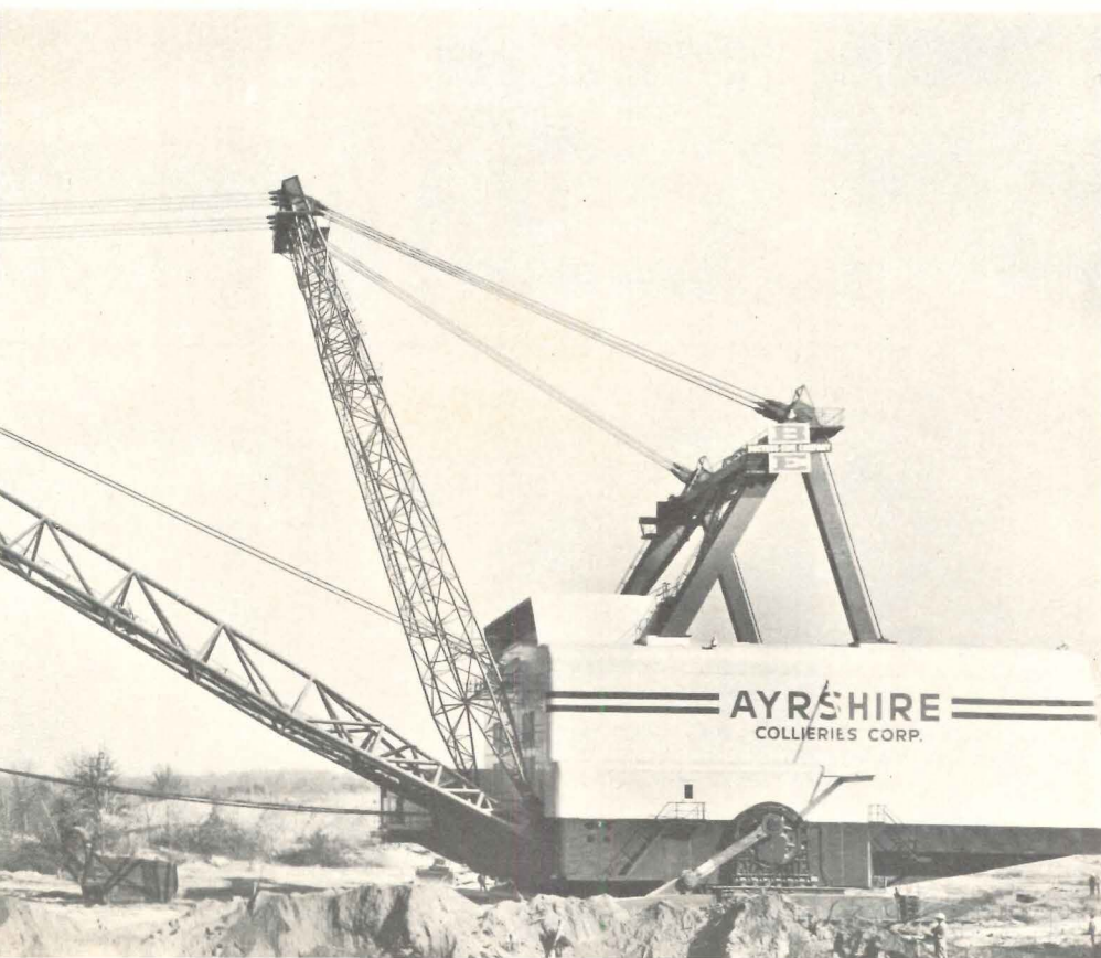
Right: Clamshell loads dump truck. Below: Dragline digs 112 tons with each cast. Lower right: Three cranes with clamshell buckets, a backhoe, and a truck work in close quarters on a crowded city site.
