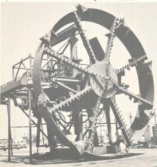
Above: Pilot bit will anchor cutter head of hard-rock mole against the tunnel face. Below: Soft-ground tunneler.
