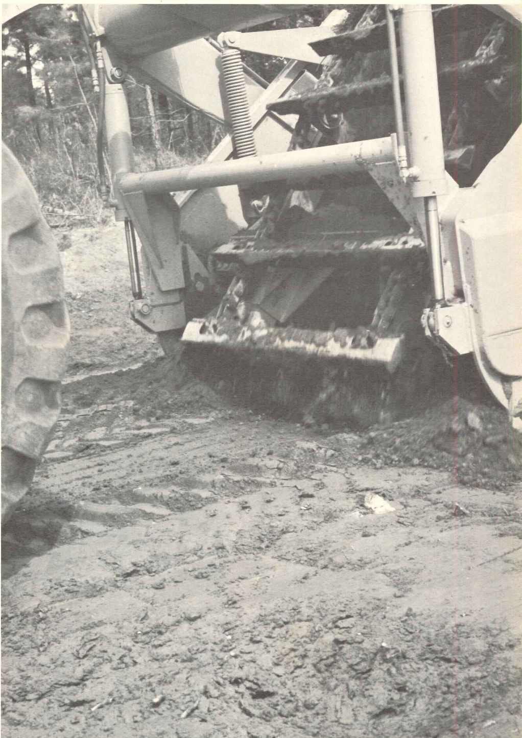
Paddle mechanism on self-loading scraper digs and lifts earth into the bowl.
