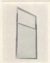
Insulated windows. Two hermetically sealed panes of glass are separated by a dehydrated airspace housing a louver screen that regulates the entrance of solar heat. By controlling the solar heat, unit helps keep air-conditioning costs down. Louvers rotate 180° and are finished with a vinyl enamel said to reflect sunlight. Thermalouver, Inc., P.O. Box 95, Flat Rock, Mich. 48134.
