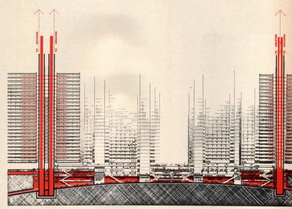
Elevation shows connections between subways and elevators.
