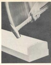
Indestructible lights. "Break/Proof" fluorescent lighting fixture is intended primarily for use in schools and institutions. The diffuser is made of highly transparent polycarbonate sheets, said to resist impacts 250 times as great as safety glass of the same thickness; these sheets are given a "self-extinguishing" rating by the ASTM. The body is hard-baked white enamei. Peerless Electric Co., 576 Folsum St., San Francisco, Calif. 94105. Circle 120, Readers' Service Card
