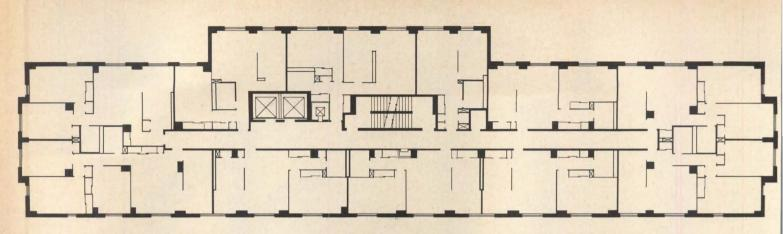
Prefabricated loadbearing wall construction (below) can easily be adapted for a New York City low-income housing project (above).
