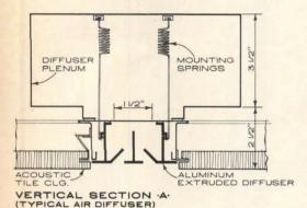
IB GA. FORMED METAL CEILING CHANNEL
