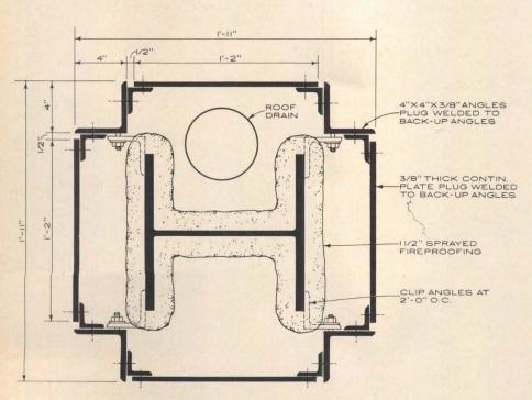
PLAN SECTION OF TYPICAL EXTERIOR COLUMN
