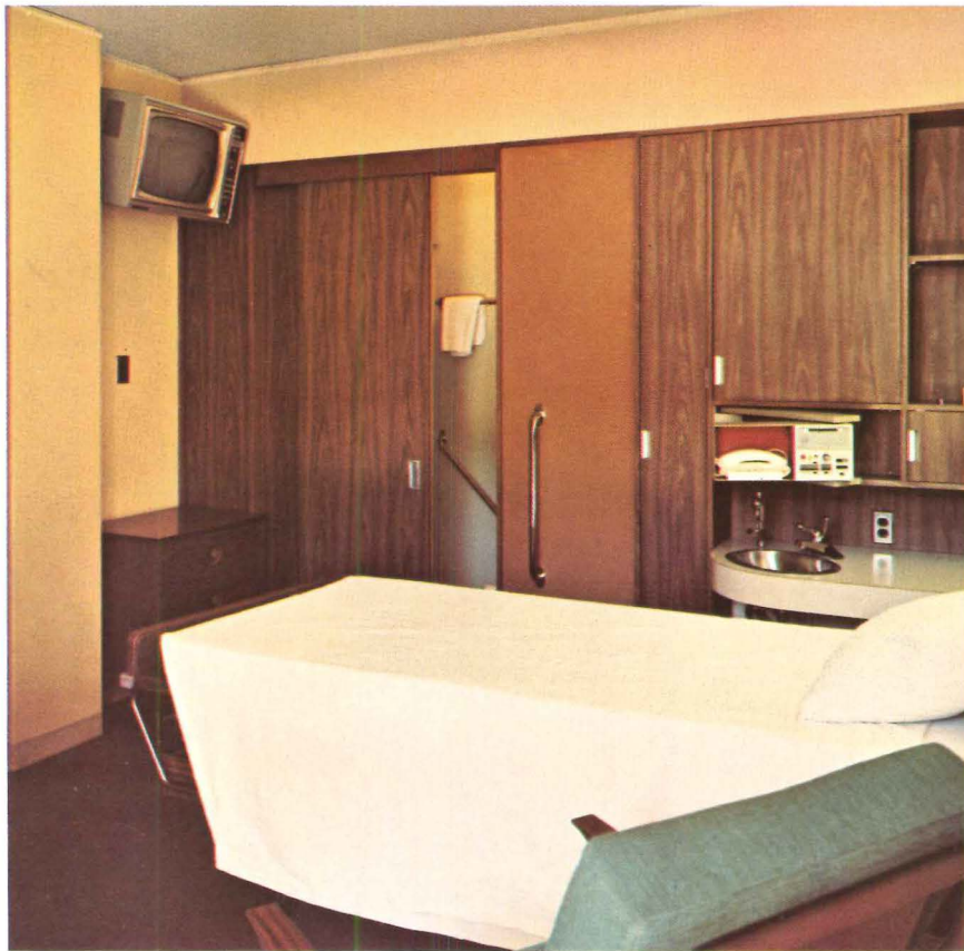
Bedside electrical console provides patients with a nurse call, telephone, TV, lighting, and curtain controls.
