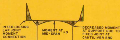
Fig. 3. Rigid frame diagram with supports moved in for floor and walls.
