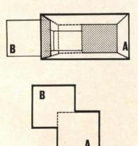
13 Overlapped spaces. From A, space completes as rectangle and is dominant over B. From B, the action is reversed.
