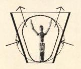
7 Sensation of space. Planes inclined in section (l.) can give a sense of uplift or depression. Planes inclined in plan (r.) can impel the body forward or imply a restraint to movement.
