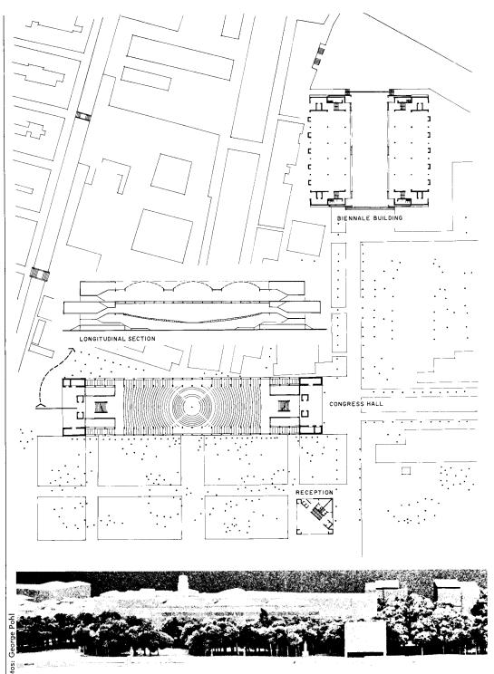
ing foundations will be carried to bed rock, if necessary. Kahn believes that each end foundation will not be required to sustain a greater load than that of the campanile in the piazza of San Marco. Reinforced concrete --long a Kahn trademark ---with marble details will be the basic construction materials.
