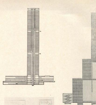
(3) The first double-deck elevator system was installed in a 60-story New York City building in 1932. Top car of each pair stopped at even-numbered floors; the bottom car stopped at odd-numbered floors.
