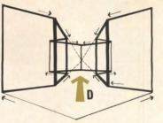
14 Square and diagonal spaces. Orientation to form is conditioned by the axis of movement. Movement on line C: form appears assymetrical; the two square spaces are linked by a diagonal passageway. Movement on line D: form appears symmetrical; two diagonal spaces are linked by a straight passageway.
