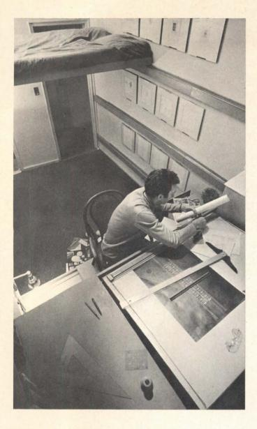
His systems-furniture for these multiple functions is a layered series of three floating, room-width platforms that slide on wall-hung rails from one end of the room to the other. Conventional ball-bearing casters mobilize the plywood platforms, which Hollander calls "trays."
