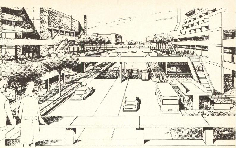
Multi-level pedestrian-motor traffic separation
