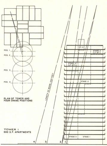
CRANE POSITIONS AND ERECTION SEQUENCE FOR TOWER I
