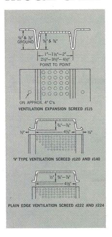
Get neater appearance, more durability with Superior ventilation expansion screed. Install in attic spaces, arcades, canopies, corridors; around eaves, foundations. Made of galvanized steel . . . also available in zinc and aluminum. Special trim available. For immediate information, phone 415 591-4461 (Belmont, Calif.). Or, write Electrical Division, H. K. Porter Company, Inc., Porter Building, Pittsburgh, Pa.
