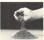
Aggregate is Celramic nodules of sealed closed-cell glass.
