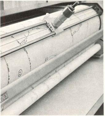
On drum plotters, such as this CalComp 763, lines in the X and Y directions are produced by lateral pen movement and
