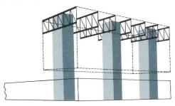
Diagram shows the cantilevered trusses and suspension system of the office tower.
