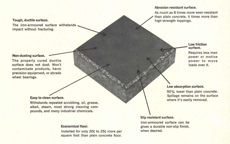
Masterplate is a specially processed metallic aggregate combined with a high-strength cement binder. Applied as a dry shake over freshly floated concrete, it produces a high-strength "iron-armoured" surface about 1/8" thick. Masterplate should be used when constructing new industrial floors or when resurfacing or replacing costly worn-out floors. For more details, call your local Master Builders field man, or write Master Builders, Cleveland, Ohio 44118.
