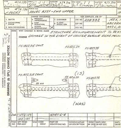
This exterior panel assembly was designed by a structural engineer on an IBM 2250 scope and was drawn on Mylar by a tape-driven X-Y Plotter. Courtesy, Lockheed-California Co.
