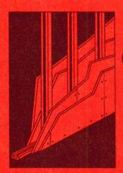
Here's a system that's both fast and simple. It gives you a quality wall with high sound-resistance (STC 45-50) and a one-hour fire-resistance rating (send for specs).
