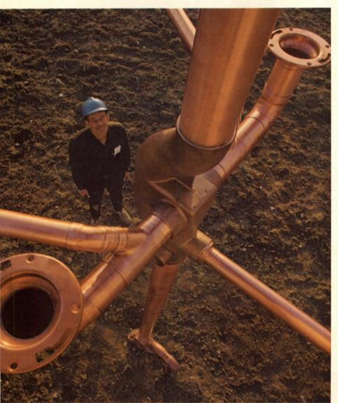
Sovent systems can be designed in 3" diameter for low rise buildings and in 4" diameter for high rise buildings. In either case the builder can expect savings over conventional drainage systems.
