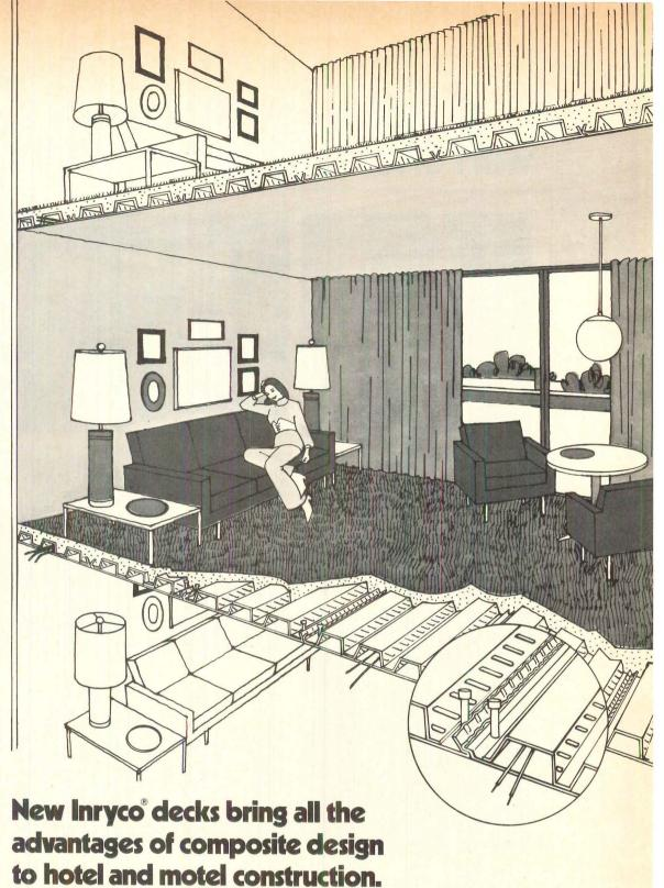
Inryco Types V, NFv and HFv Floor/Ceiling systems make possible long span composite slabs that create spacious uninterrupted areas. The smooth underside of the deck is treated to accept a sprayed-on finish that looks like plaster, and eliminates the need for suspended ceilings and the extra building height they require. In addition, floor cells can carry electrification for rooms above and below. And recent UL Ratings often make it possible to eliminate costly fireproofing.
