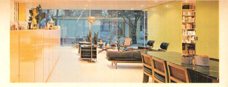
Clean look of living-dining area, above, and bedroom, below, is achieved through lack of wall moulding, self-leveling polyurethane floor and suspended ceilings separated only by steel bents. Kitchen opens directly to dining area; rear façade, far left, has glass panels like the front.
