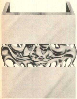
Now the temperature drops. By 9:00 p.m. it is 20°; the joint opens up to  $\frac{7}{16}$ ". And while the job called for a 3/8" cured bead that could move 25% either way, it actually winds up with a 1/4" cured bead that must elongate more than 50% to  $\frac{7}{16}$ ". It probably won't stick it out. (Above, right).
