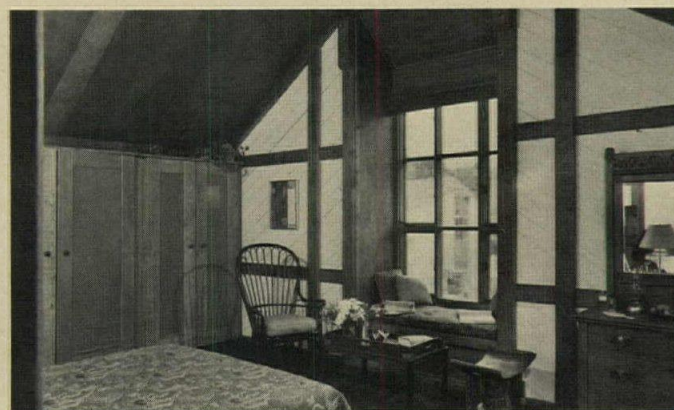
Severe exterior of largely prefabricated Amherst Fields housing conceals wealth of interior configurations. Post and beam framing is strong context for interior design. Photos: Ezra Stoller © ESTO.
