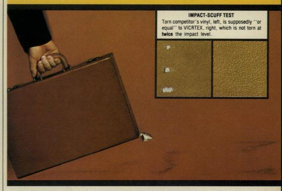
Most tears in wallcoverings result from a glancing blow occurring on a plane parallel to the floor — such as by an attache case, shown above.
