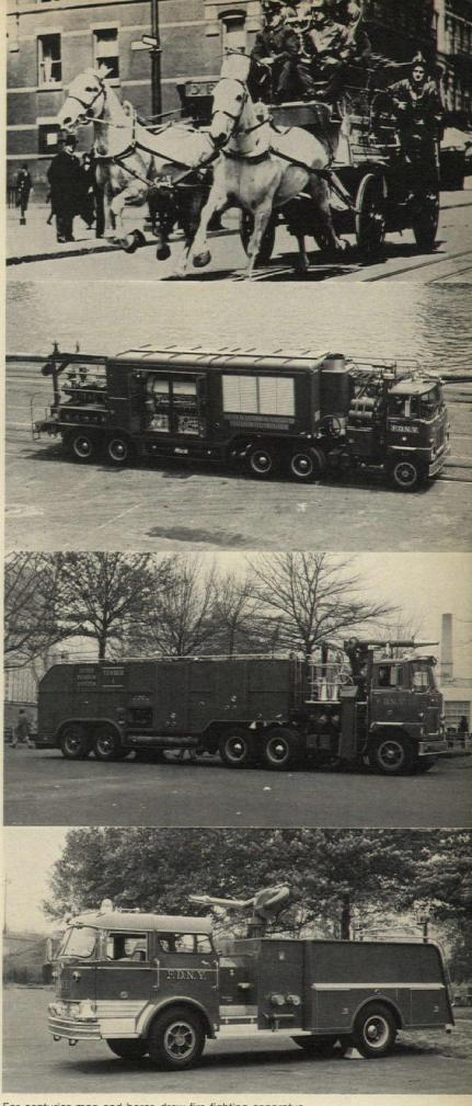
For centuries man and horse drew fire fighting apparatus. Today, New York City alone employs advanced super pumper system: super pumper (diesel pump), tender (carries large diameter hose) and satellite (for large caliber streams). Photography: Fire Dept. of New York Photo Unit.
