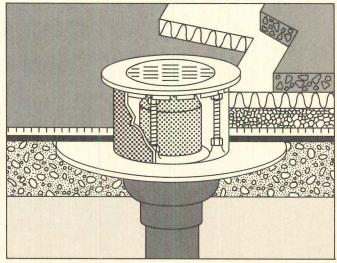
If you're designing a poured concrete wearing slab, our unique All-Level Drain used with TREMproof assures positive drainage on all levels. Water is taken off the traffic surfaces, the insulation layer, the percolation layer, and the waterproofing layer itself.
