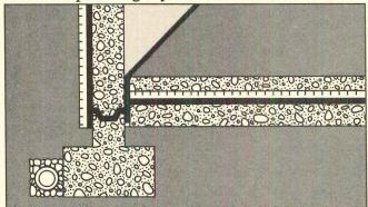
Of course TREMproof liquid polymers can be used for the waterproofing of foundations, planters, reflecting pools, etc. They're selfadhering and become an integral part of the
