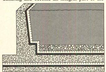
structure. Their superior adhesive quality prevents any lateral movement of water between the substrate and waterproofing blanket.
