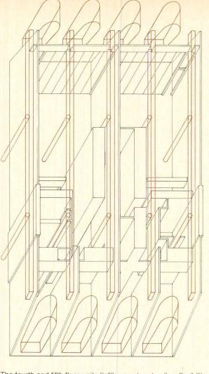
The fourth and fifth floor units (left) are set up to allow flexibility in the number of bedrooms by changing the location of a single panel. The fusion of three systems in the reuse scheme is seen as important in itself: The existing loft structure, the town house plan and the early "modern" idea of separating structure and screening (illustrated in the drawing above). All combine to denote a schism between old and new while commenting on the continuity of architecture and urbanism.
