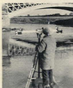
Two instruments of photogrammetry. (Above left) photographer positions stereometric camera. (Above right) operator tends plotting instrument.
