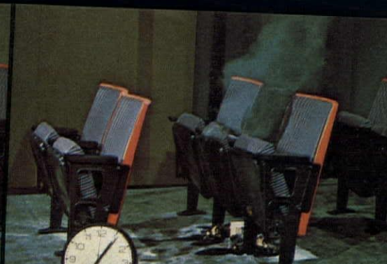
Major flames out. Time: 6 minutes, 00 seconds. Damage: 1 chair involved, fabric melting and smoldering on two adjoining chairs.
