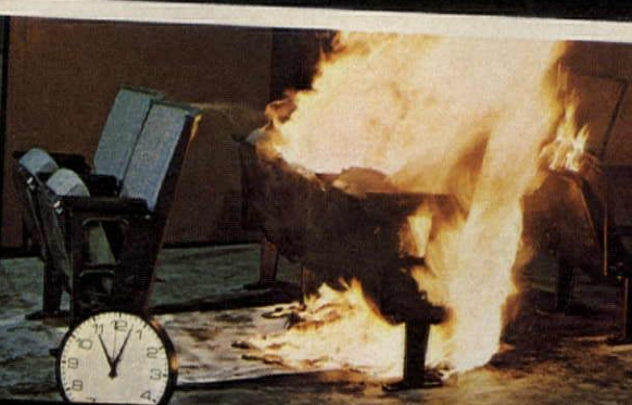
Time: 3 minutes, 00 seconds. Five chairs in two rows involved.
