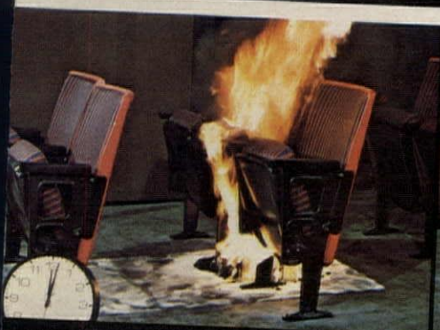
TEST TWO: HR POLYURETHANE containing flame retardants. Time: 1 minute, 30 seconds after ignition.
