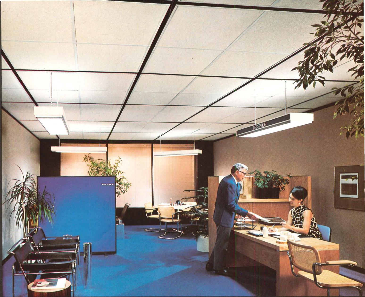
This pendant fixture, movable to many points in the room, provides both quality task lighting and substantial energy savings.
