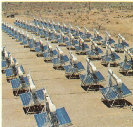
Intensive testing (EMMAQUA) conducted by Desert Sunshine Exposure Tests, Inc. in the Arizona desert has established the excellent resistance of Galbestos to color change and fade.
