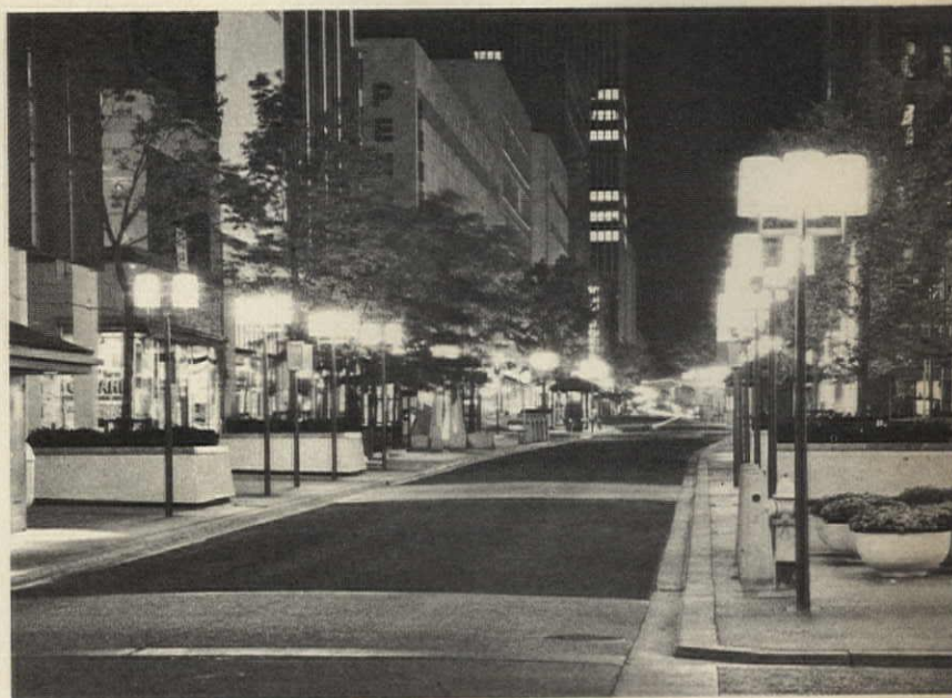
Nicollet Mall in Minneapolis (above) is illuminated by pole fixtures holding two or four plastic covers, each with eight incandescent lamps. Mercury vapor uplights on trees. Design: Seymour Evans & Associates. City Park in Highland Park, Tx (below), uses clear mercury lighting mounted in shielded fixtures hidden in the trees. Design: John Watson.
