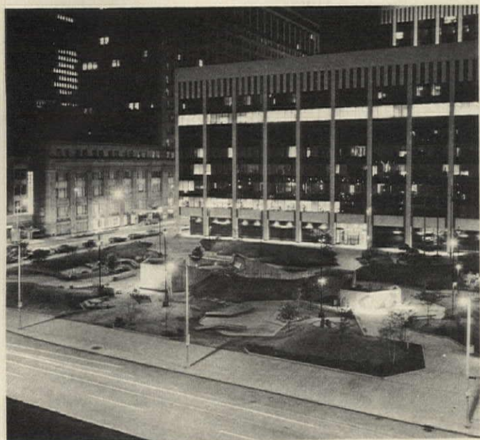
Cleveland's Chester Common, a mini-park designed to accommodate many types of activities (above and below) has mercury vapor general night time illumination. Accent lighting is with 12v incandescent lamps. Surrounding lighting is HPS. Design: P. Heintzelman, R. Reeves of the Cleveland Department of Community Development, Downtown Planning.
