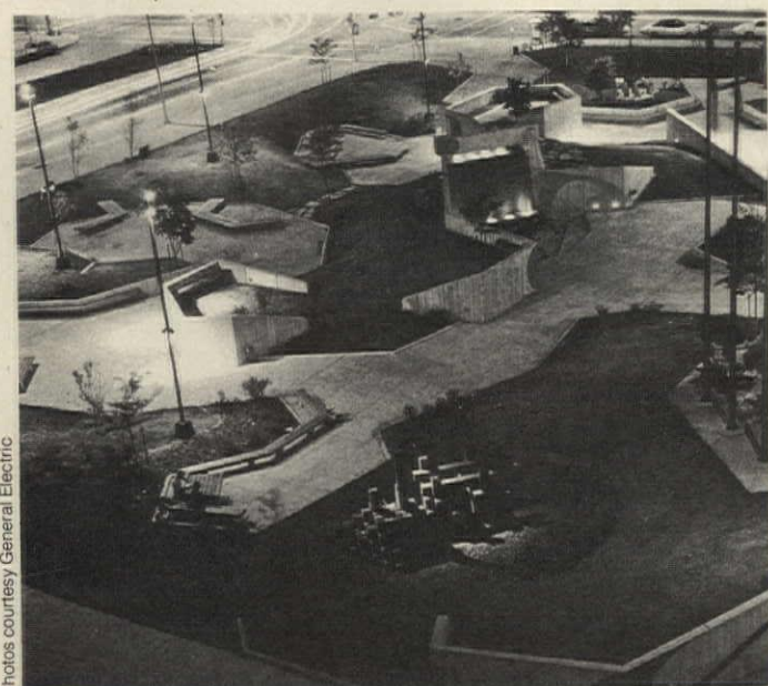
Cleveland's Chester Common, a mini-park designed to accommodate many types of activities (above and below) has mercury vapor general night time illumination. Accent lighting is with 12v incandescent lamps. Surrounding lighting is HPS. Design: P. Heintzelman, R. Reeves of the Cleveland Department of Community Development, Downtown Planning.
