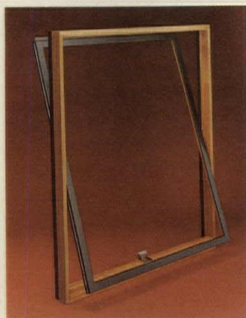
Pivot sash brings outdoor glass surface inside for fast and economical maintenance. When pivoted, the sash is held in washing position by a catch.
