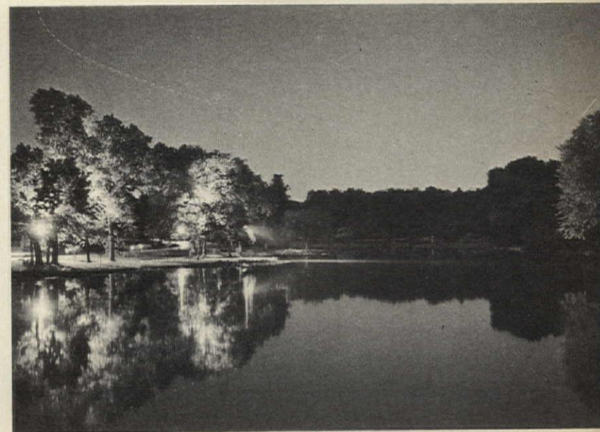
Nicollet Mall in Minneapolis (above) is illuminated by pole fixtures holding two or four plastic covers, each with eight incandescent lamps. Mercury vapor uplights on trees. Design: Seymour Evans & Associates. City Park in Highland Park, Tx (below), uses clear mercury lighting mounted in shielded fixtures hidden in the trees. Design: John Watson.
