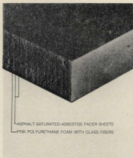
Three types of roof insulation, from left: glass fiber reinforced urethane foam with asphalt-saturated facers; polyurethane core with glass fiber reinforcing and skins of asphalt-impregnated felt; combination of polyurethane core, asphalt-felt skin, and bonded perlite lower layer
