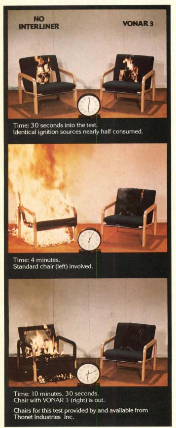
At the start of this test, these chairs were identical in every way but one. Both were made with identical 60% wool/40% polyester upholstery fabric, standard polyurethane foam in the seat and back cushions, and wood structural parts. But the chair on the right had a layer of VONAR\* 3 interliner (3/16" thickness) added as an envelope around the polyurethane foam in the back and seat cushions.
