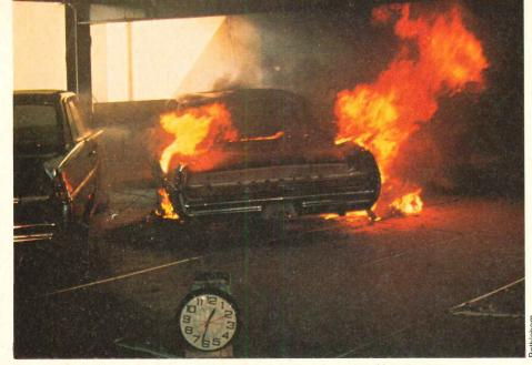
Scranton fire test to measure damage to exposed steel in a typical parking structure.
