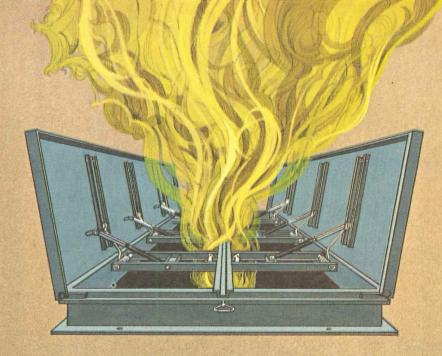
**Big Smoky**<sup>M</sup> – **Heat and Smoke Vents for 5' 0**, **5' 6 and 6' 0 Joist Spacings.** The first automatically operating Heat and Smoke Vent available in economical steel onstruction in widths to span wide joist spacings...permitting installation without special supplemental aming. Furnished in lengths from 6'0" thru 12'0". Underwriters` Laboratories listed and Factory Mutual pproved. Also available in aluminum.
