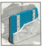
Apply over exterior masonry or concrete walls with metal "Z" channels or wood furring strips. Finish with lath and stucco.
