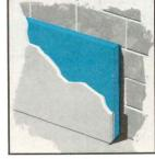
Apply over interior masonry or concrete walls with STYROFOAM brand insulation mastic No. 11. Finish with gypsum wall board.
