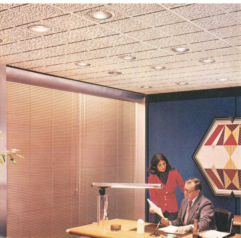
handsome rough-textured 24" x 48" panel is scored in both directions with one-inch-wide routings that divide the surface into eight tilelike sections. Second Look I, with its smoother surface, is also divided to simulate 12" x 12" tile, while Second Look II provides the broader look of a 24" x 24" tegular-edge panel.
