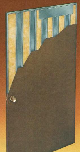
747 Series. 747 Series. Extra heavy-duty door, recommended for factories, work areas, shipping or receiving locations, etc. Available in any thickness, height, widths up to 5'. Steel-ribbed, with either cold rolled or galvanealed 14-, 16- or 18-gauge face skins. Like 707 Series, utilizes U-shaped, hinged reinforcing channel and a continuous, beveled ½-inch in 2-inch lock edge channel in 2-inch lock edge channel.
