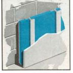
Apply over exterior masonry or concrete walls with metal "Z" channels or wood furring strips. Finish with metal or wood exterior siding.
