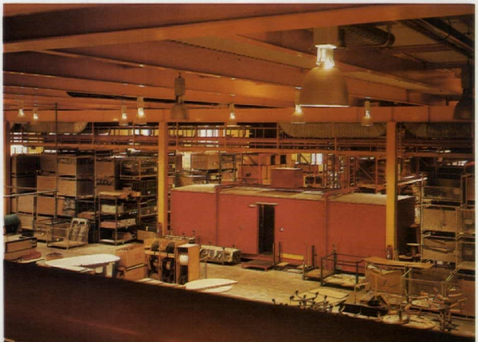
Internal flexibility is important in the open-plan factory; all main services are reached from a centrally located overhead catwalk (above); and toilet stalls (below and left) are portable.
