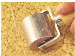
Chemically welded seams help to protect against penetration of moisture and dirt
