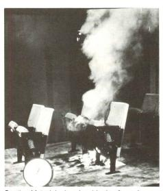
Seating Materials, Inc. (cushioning foams) show the comparative flammability of standard polyurethane foam cushioning (left) and the much lower flammability of neoprene foam cushioning (right) under identical conditions.
