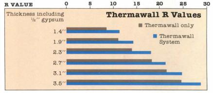
Our unique Thermawall Fastening System (patent pending) eliminates common studs and batt insulation. It's thinner than conventional stud walls, so you gain floor space. And at the same time solve an old problem of increasing square footage for tenants.
