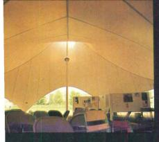
The logic of this tensioned membrane structure is as exciting as its appearance. A canopy over a school yard play area, it provides shelter for outdoor activities in almost any weather. The attractive "upsidedown" design allows rain water runoff through the support columns.
